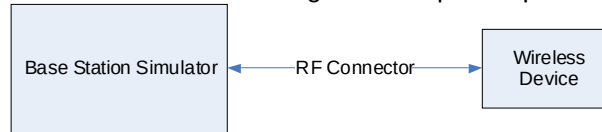
Figure 9-2 Power Measurement Setup
