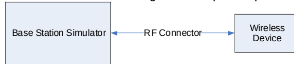
Figure 9-2 Power Measurement Setup
