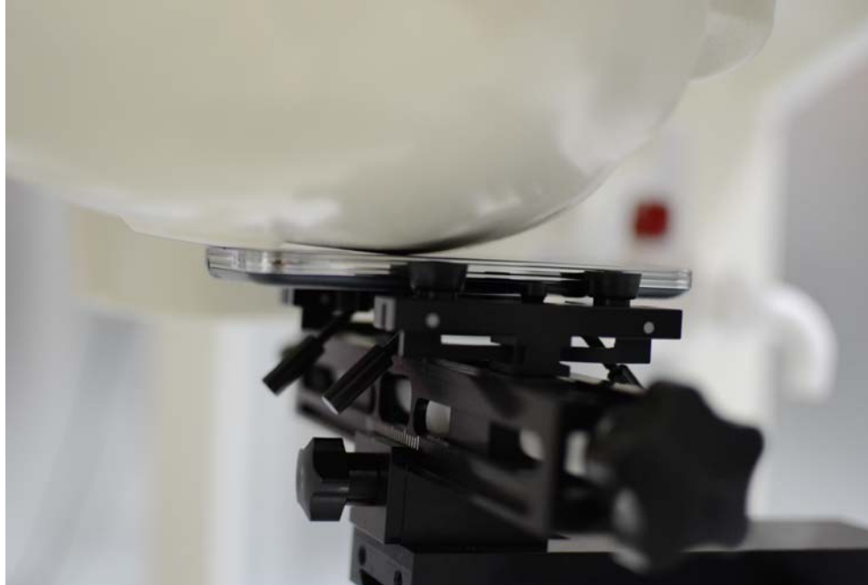
SAR Test Setup Photo 1 – Right Cheek
