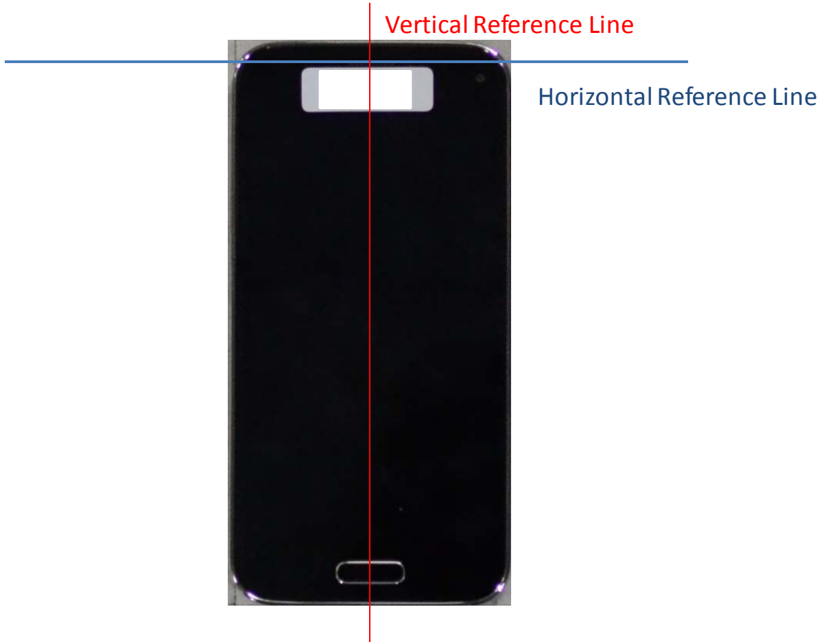
SAR Test Setup Photo 11 – Horizontal and Vertical Reference Lines
