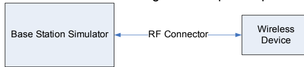
Figure 9-2 Power Measurement Setup
