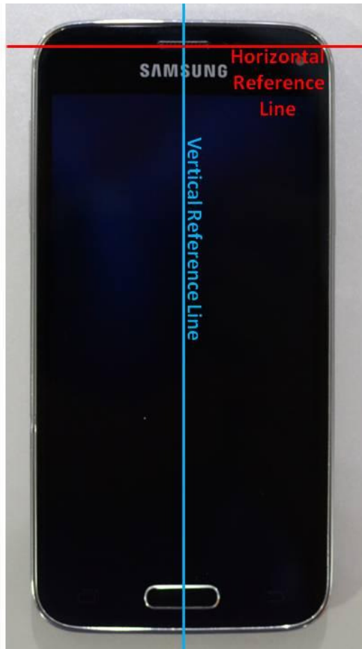
SAR Test Setup Photo 11 – DUT Reference Lines
