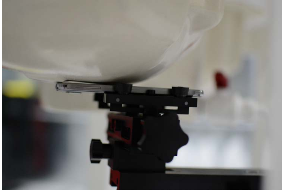
SAR Test Setup Photo 1 - Right Cheek
