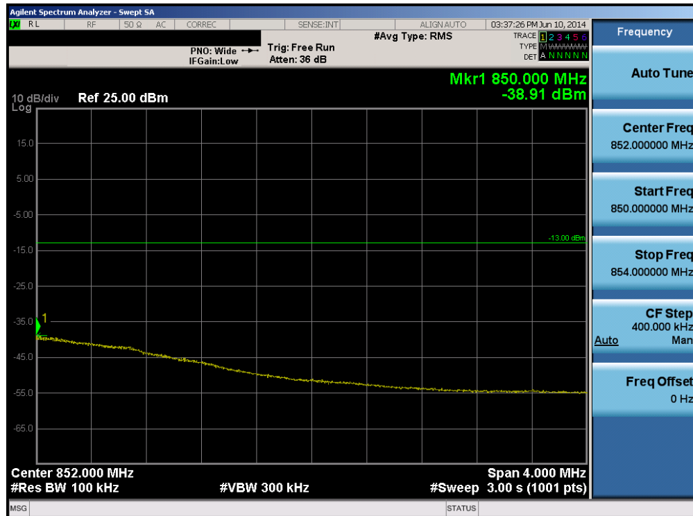
Plot 6-36. Upper Extended Band Edge Plot (Band 5 – 1.4MHz QPSK – RB Size 6)
