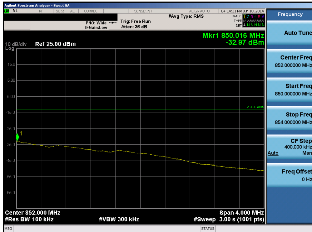
Plot 6-44. Upper Extended Band Edge Plot (Band 5 - 5.0MHz QPSK - RB Size 25)
