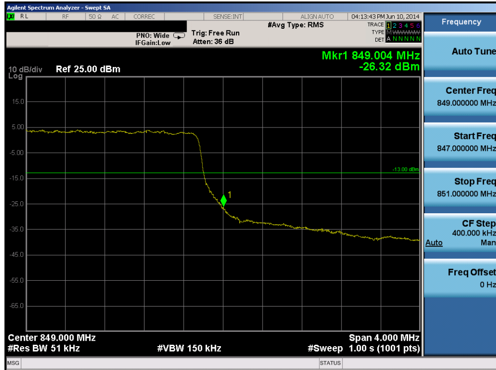
Plot 6-43. Upper Band Edge Plot (Band 5 - 5.0MHz QPSK - RB Size 25)
