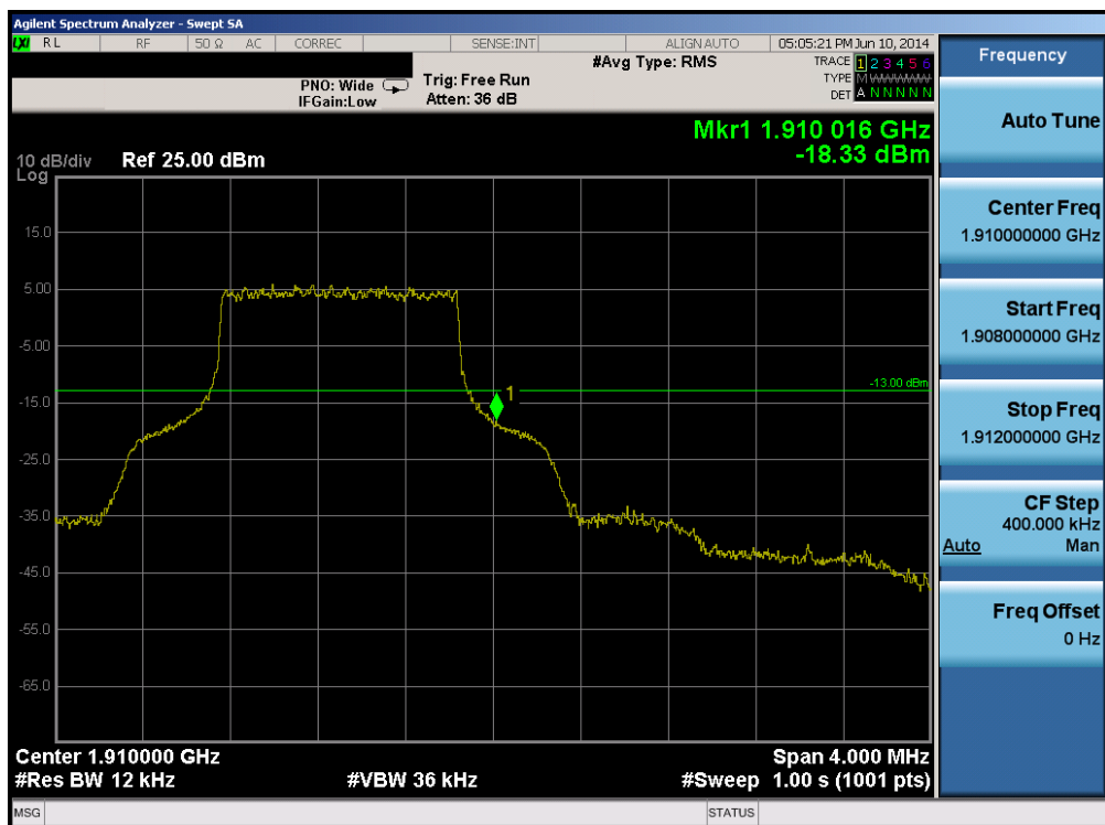
Plot 6-49. Upper Band Edge Plot (Band 2 – 1.4MHz QPSK – RB Size 6)
