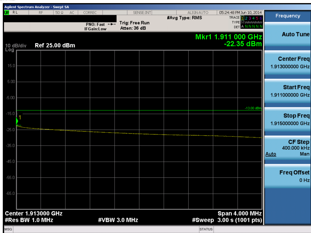
Plot 6-62. Upper Extended Band Edge Plot (Band 2 – 10.0MHz QPSK – RB Size 50)
