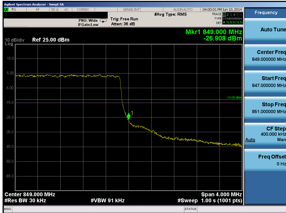
Plot 6-39. Upper Band Edge Plot (Band 5 - 3.0MHz QPSK - RB Size 15)
