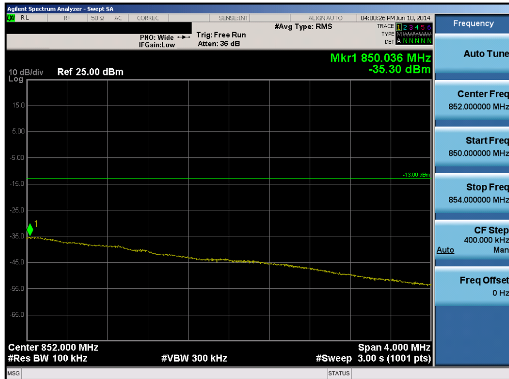
Plot 6-40. Upper Extended Band Edge Plot (Band 5 - Band 5 - 3.0MHz QPSK - RB Size 15)
