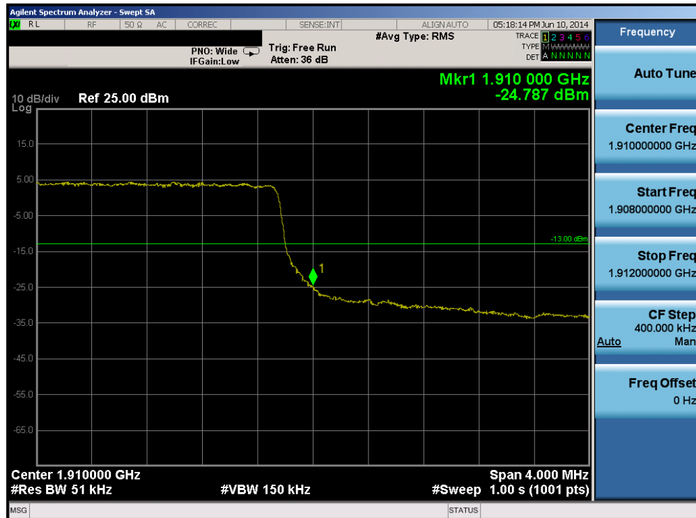
Plot 6-57. Upper Band Edge Plot (Band 2 – 5.0MHz QPSK – RB Size 25)
