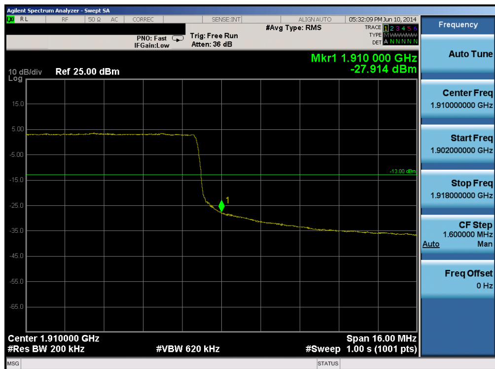
Plot 6-69. Upper Band Edge Plot (Band 2 – 20.0MHz QPSK – RB Size 100)
