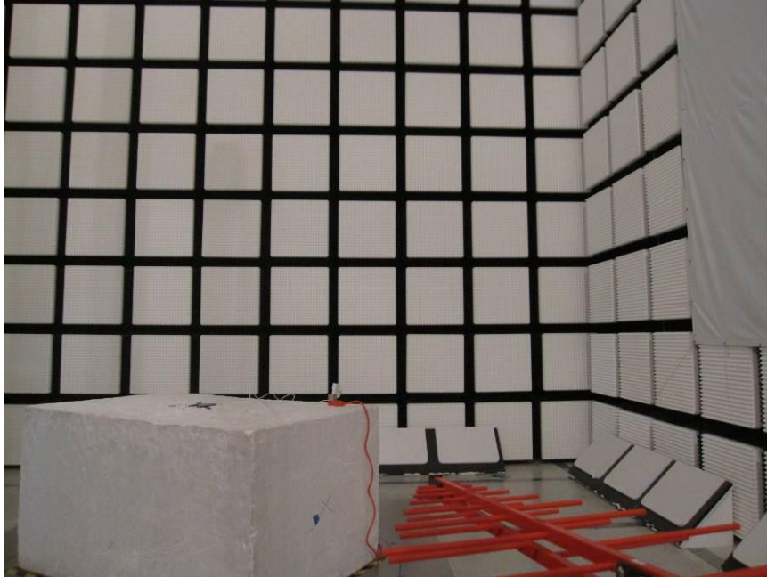
RADIATED FRONT PHOTO (BELOW 1 GHz)
