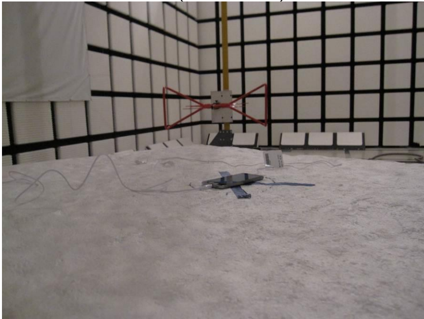
RADIATED BACK PHOTO (BELOW 1 GHz)
