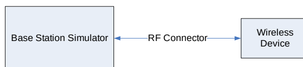
Figure 9-2 Power Measurement Setup
