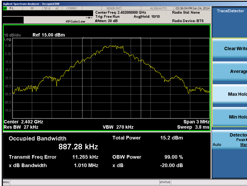
Plot 6-1. 20dB Bandwidth Plot (Bluetooth, 1Mbps – Ch. 0)
