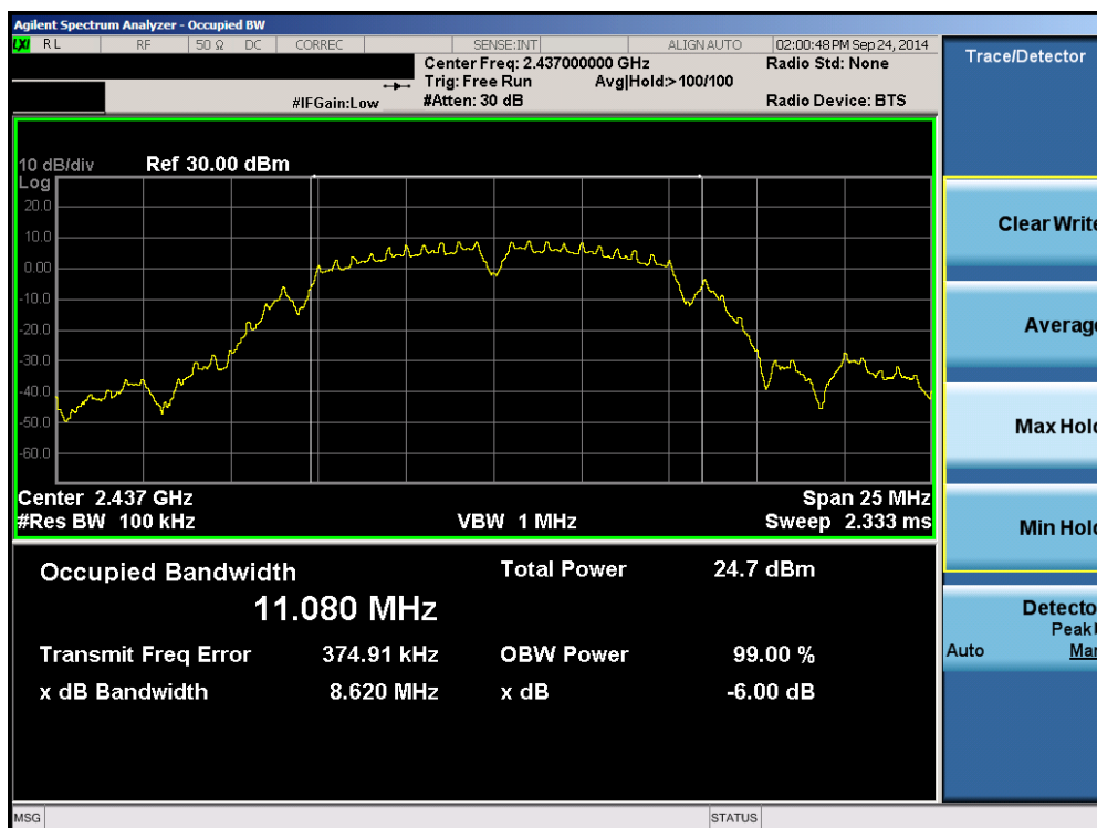
Plot 6-2. 6dB Bandwidth Plot (802.11b – Ch. 6)
