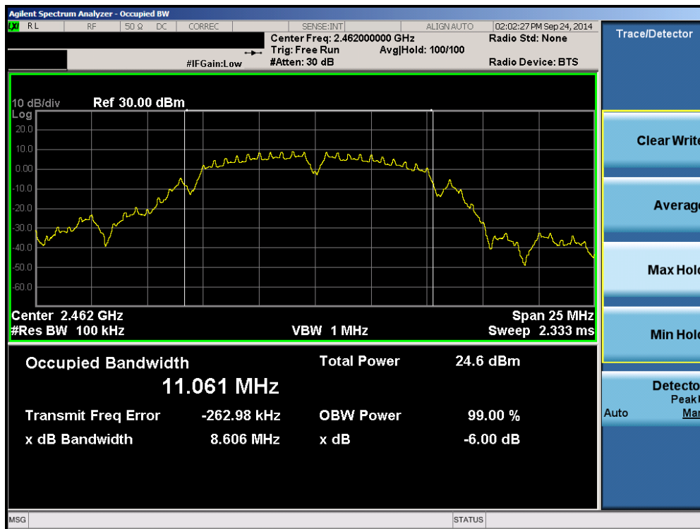
Plot 6-3. 6dB Bandwidth Plot (802.11b – Ch. 11)
