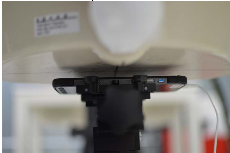
SAR Test Setup Photo 6: Back Side at 10 mm with Headphones
