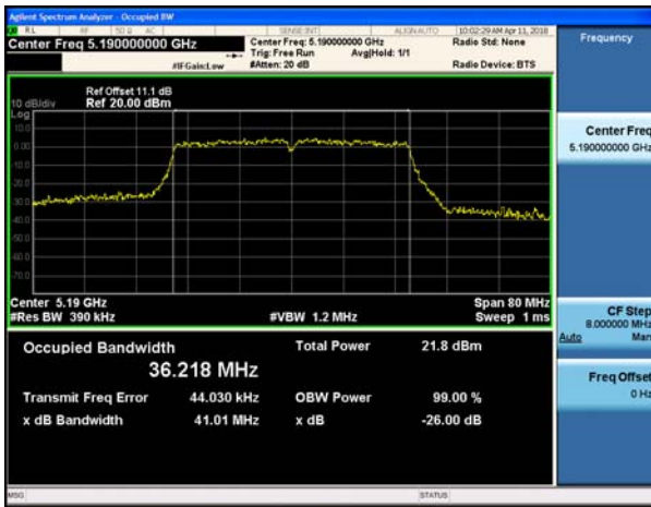
802.11ac_VHT40 UNII 2C BAND 26dB Bandwidth(CH 118)
