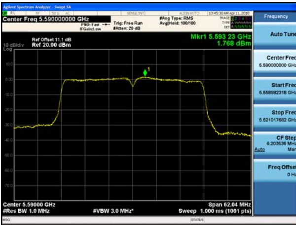
802.11ac_VHT40 UNII 2C BAND PSD CH 118
