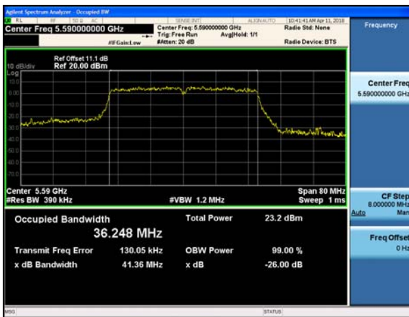
802.11ac_VHT40 UNII 2C BAND 26dB Bandwidth(CH 118)
