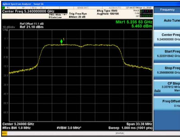
802.11n_HT20 UNII 2C BAND PSD CH 120
