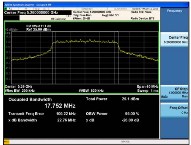
802.11ac_VHT20 UNII 3 BAND 26dB Bandwidth(CH 165)
