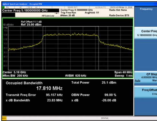
802.11ac_VHT20 UNII 2C BAND 26dB Bandwidth(CH 140)
