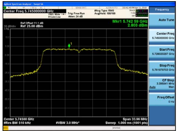
802.11n_HT20 UNII 3 BAND PSD CH 149
