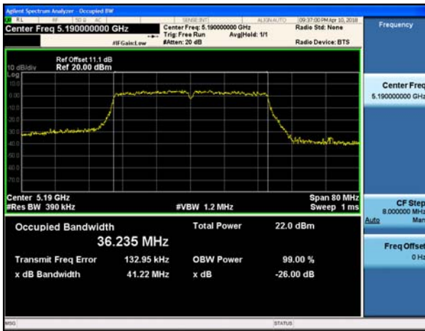
802.11n_HT40 UNII 2C BAND 26dB Bandwidth(CH 118)
