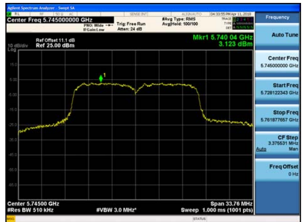
802.11ac_VHT20 UNII 3 BAND PSD CH 149
