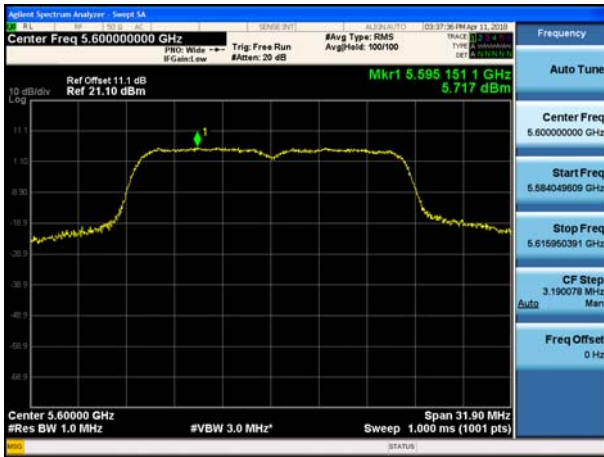
802.11n_HT20 UNII 2C BAND PSD CH 120
