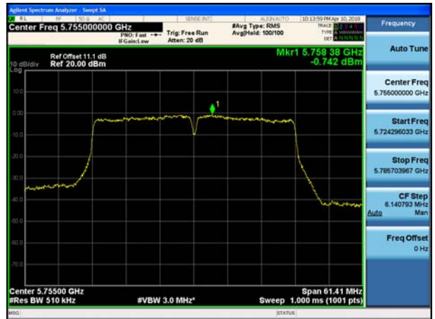
802.11n_HT40 UNII 3 BAND PSD CH 151
