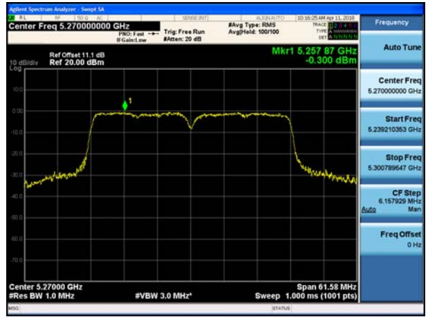
802.11ac_VHT40 UNII 3 BAND PSD CH 159
