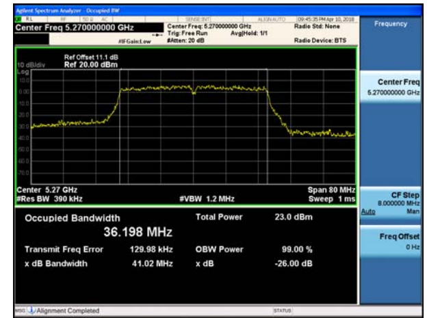
802.11n_HT40 UNII 3 BAND 26dB Bandwidth (CH 159)
