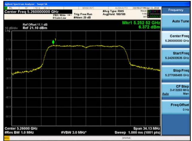
802.11ac_VHT20 UNII 3 BAND PSD CH 149
