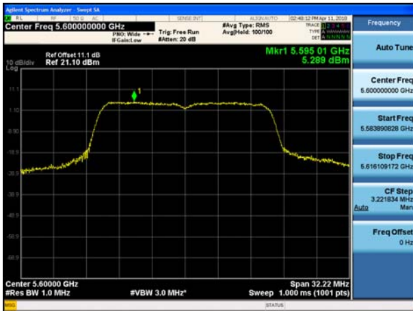
802.11a UNII 2C BAND PSD CH 120
