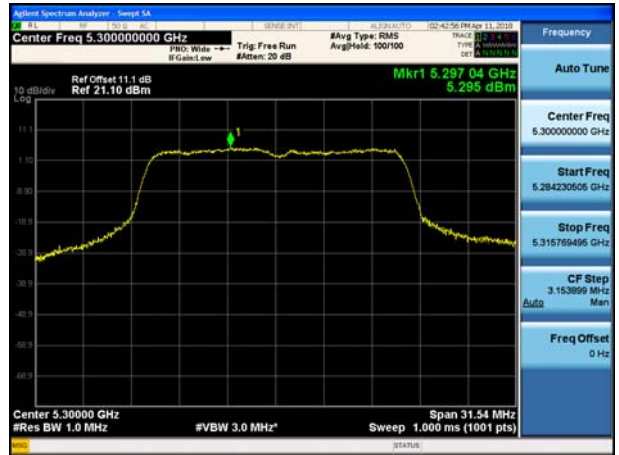
802.11a UNII 3 BAND PSD CH 149
