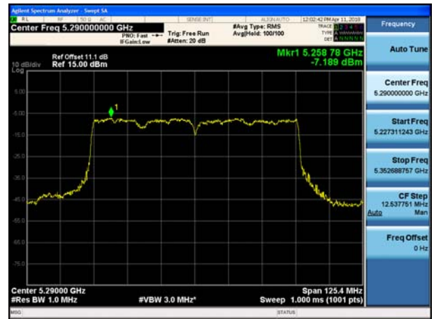
802.11ac_VHT80 UNII 3 BAND PSD CH 122
