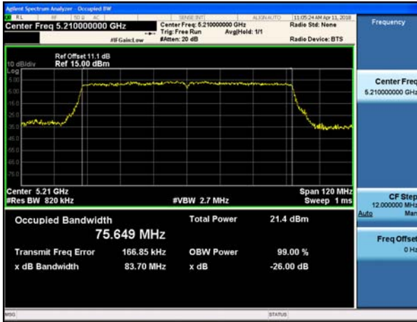
802.11ac_VHT80 UNII 2C BAND 26dB Bandwidth(CH 106)
