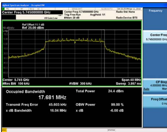
802.11ac_VHT20 UNII 3 BAND 6dB Bandwidth(CH.149)
