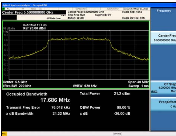
802.11n_HT20 UNII 2C BAND 26dB Bandwidth(CH 100)
