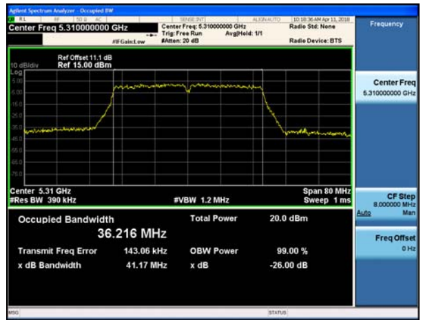
802.11ac_VHT40 UNII 3 BAND 26dB Bandwidth (CH 159)
