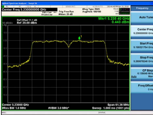
802.11n_HT40 UNII 2C BAND PSD CH 134
