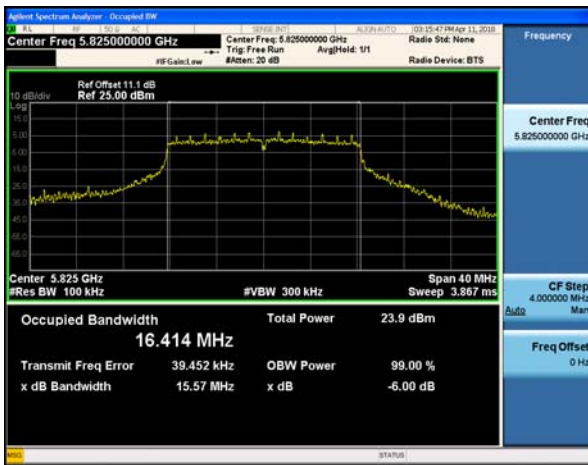
802.11ac_VHT20 UNII 3 BAND 6dB Bandwidth(CH.149)
