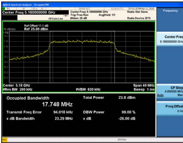
802.11n_HT20 UNII 2C BAND 26dB Bandwidth(CH 100)
