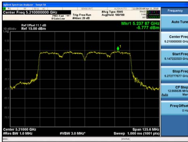
802.11ac_VHT80 UNII 2C BAND PSD CH 106
