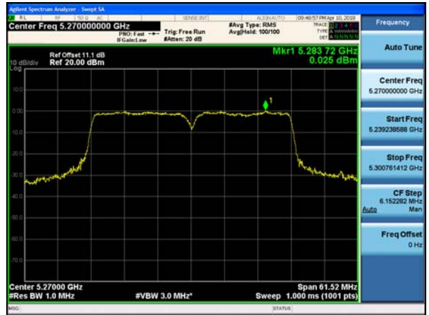
802.11n_HT40 UNII 3 BAND PSD CH 151
