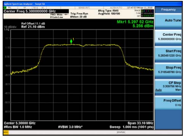
802.11n_HT20 UNII 3 BAND PSD CH 149
