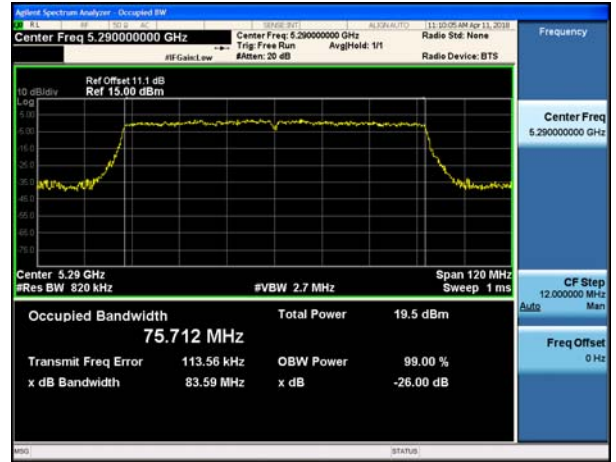
802.11ac_VHT80 UNII 3 BAND 26dB Bandwidth(CH 122)
