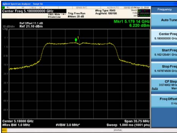
802.11ac_VHT20 UNII 2C BAND PSD CH 140
