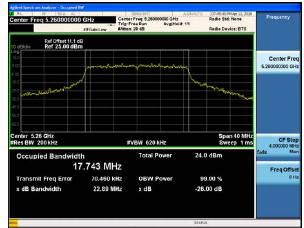
802.11n_HT20 UNII 3 BAND 26dB Bandwidth(CH 149)
