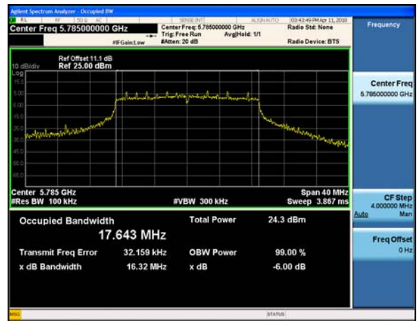
802.11n_HT20 UNII 3 BAND 6dB Bandwidth(CH.157)
