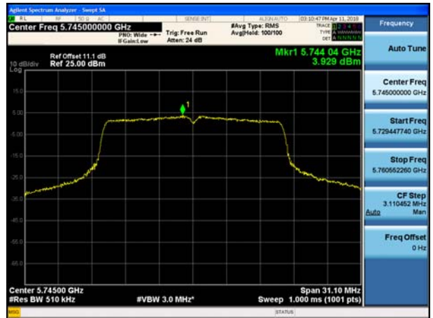
802.11a UNII 3 BAND PSD CH 149
