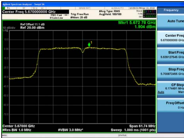
802.11n_HT40 UNII 2C BAND PSD CH 134
