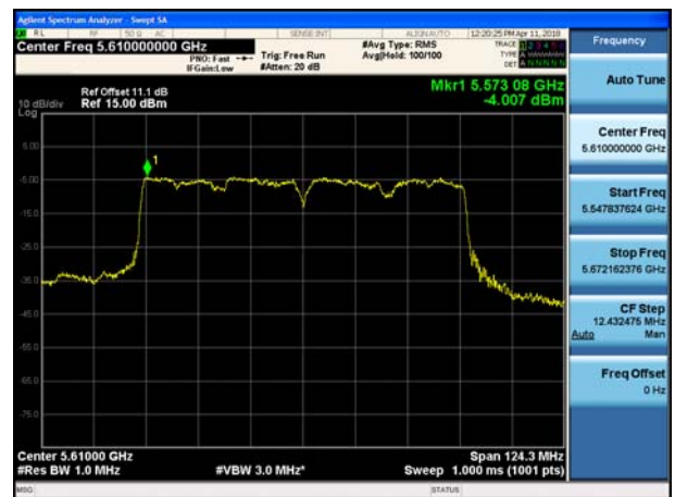
802.11ac_VHT80 UNII 3 BAND PSD CH 122
