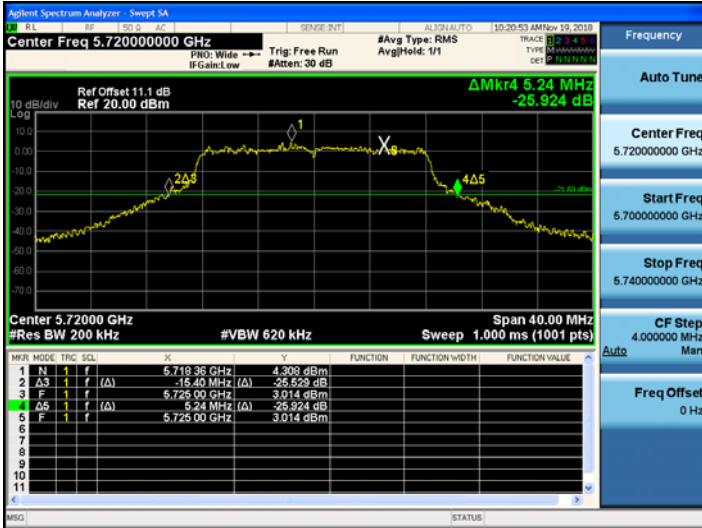
802.11ac_VHT20 CH.144 Bandwidth
