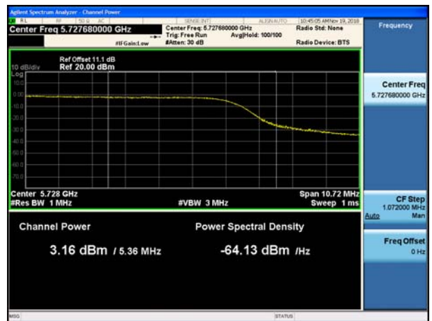
802.11ac_VHT20 UNII 3 Band Average Power CH.144
