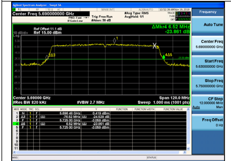
802.11ac_VHT80 CH.138 Bandwidth
