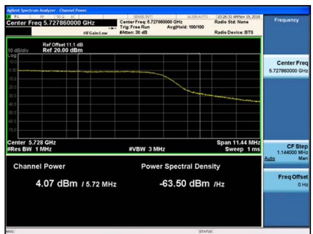
802.11ac_VHT20 UNII 3 Band Average Power CH.144
