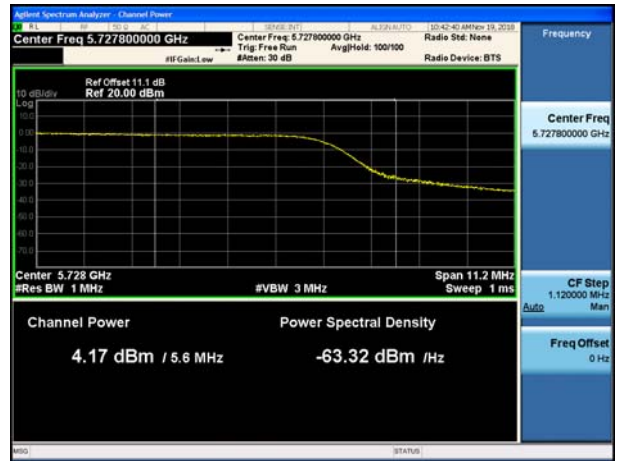
802.11ac_VHT20 UNII 3 Band Average Power CH.144
