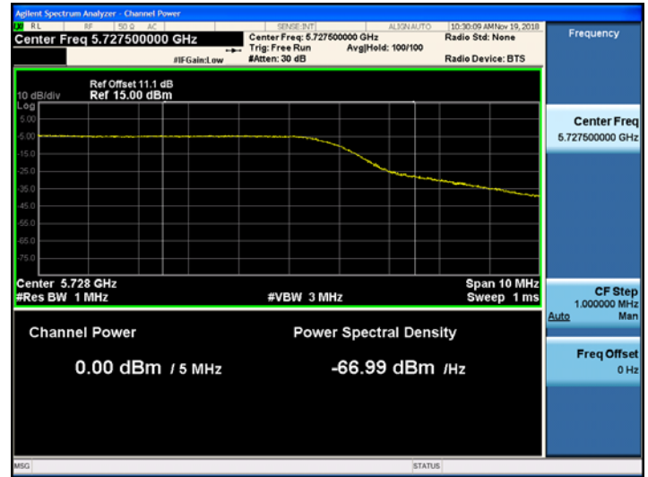
802.11ac_VHT40 UNII 3 Band Average Power CH.142
