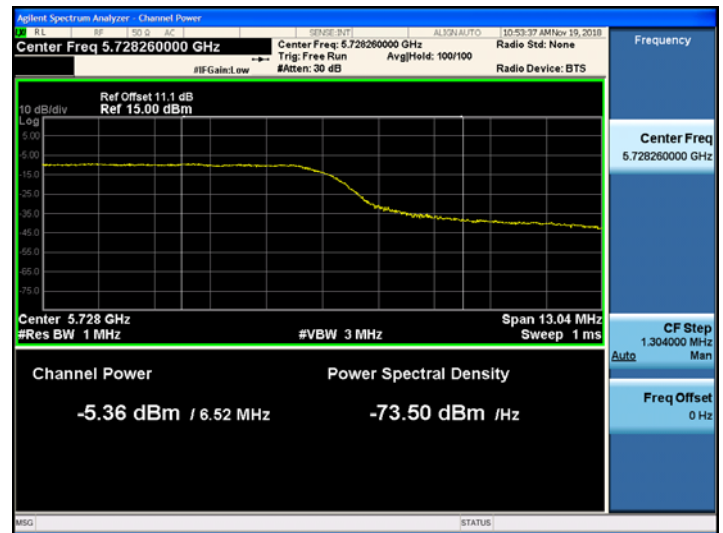
802.11ac_VHT80 UNII 3 Band Average Power CH.138
