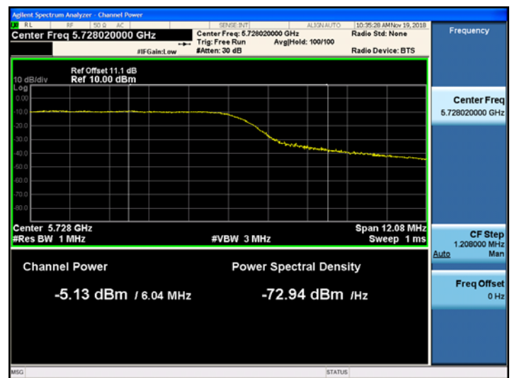
802.11ac_VHT80 UNII 3 Band Average Power CH.138
