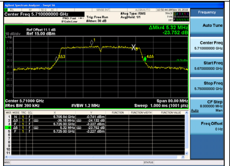
802.11ac_VHT40 CH.142 Bandwidth
