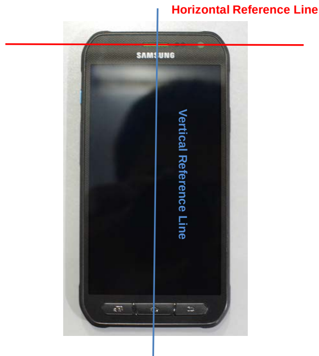
SAR Test Setup Photo 12: Horizontal and Vertical Reference Lines
