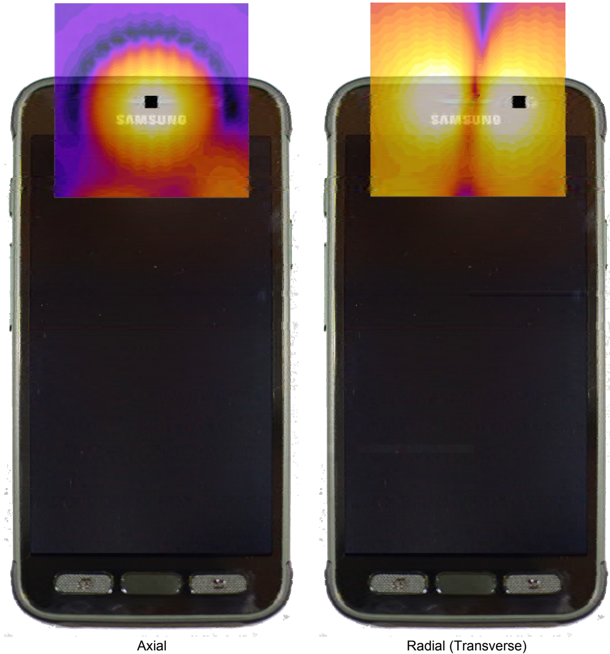
Figure 15-3 T-Coil Scan Overlay Magnetic Field Distributions
