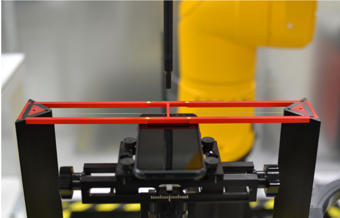
Figure 18-1 Ear Reference Point HAC Phantom Alignment
