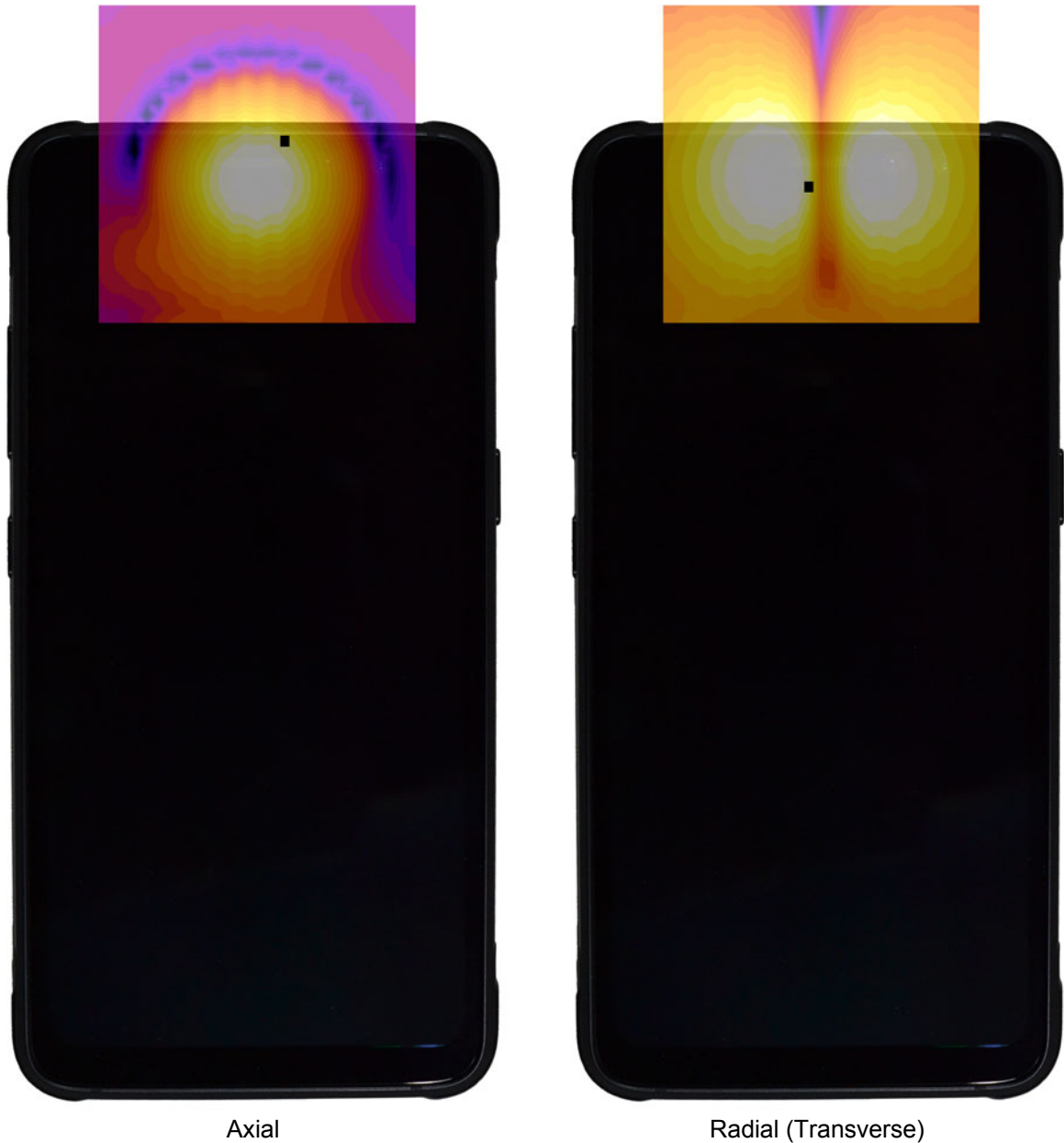
Figure 14-3 T-Coil Scan Overlay Magnetic Field Distributions
