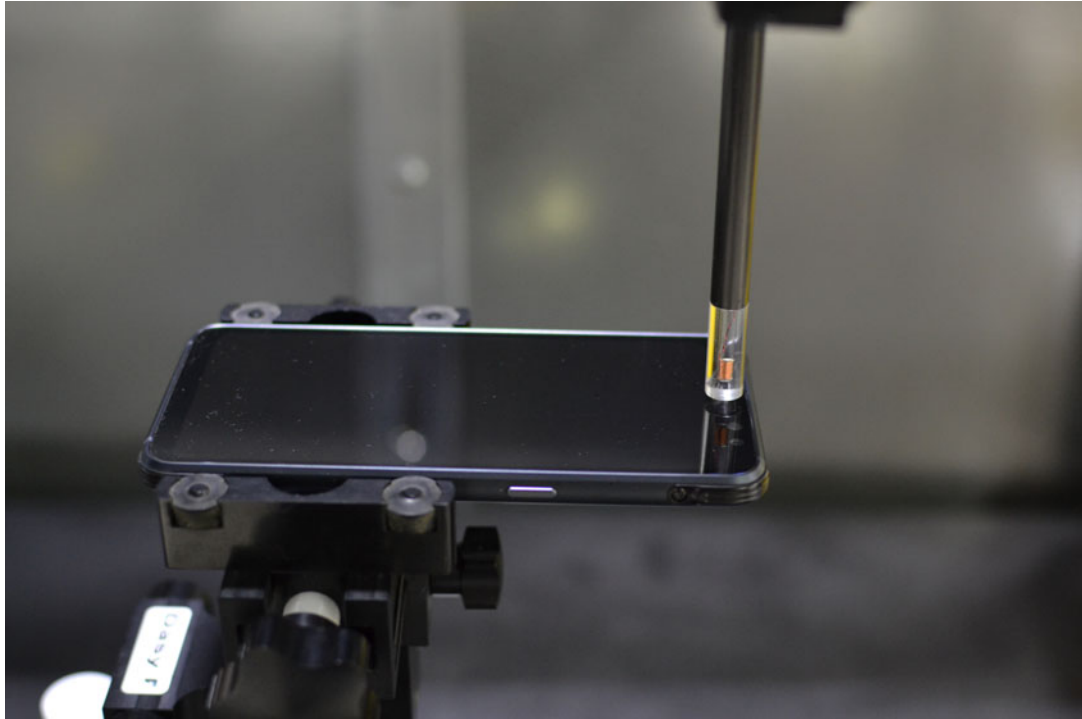
Figure 14-1 Test Setup for Wireless Device
