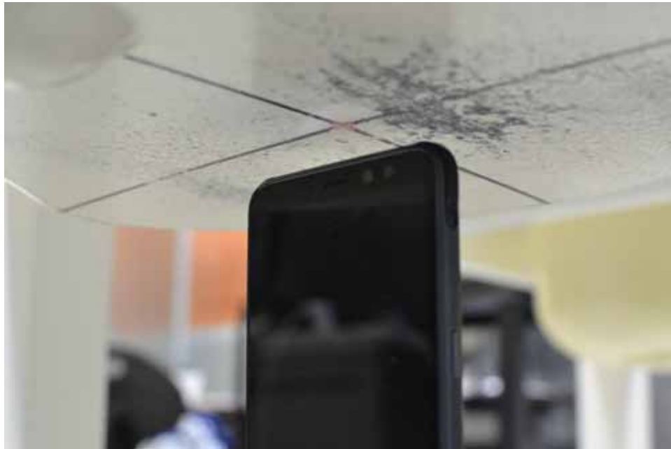
SAR Test Setup Photo 12 – Top Edge at 10 mm
