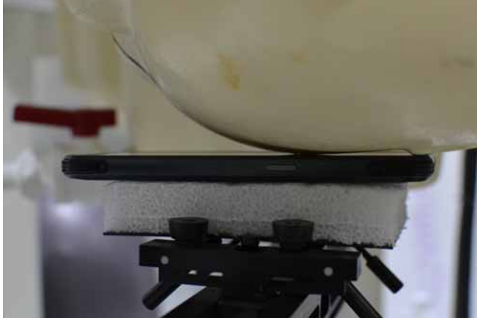
SAR Test Setup Photo 3 – Left Cheek
