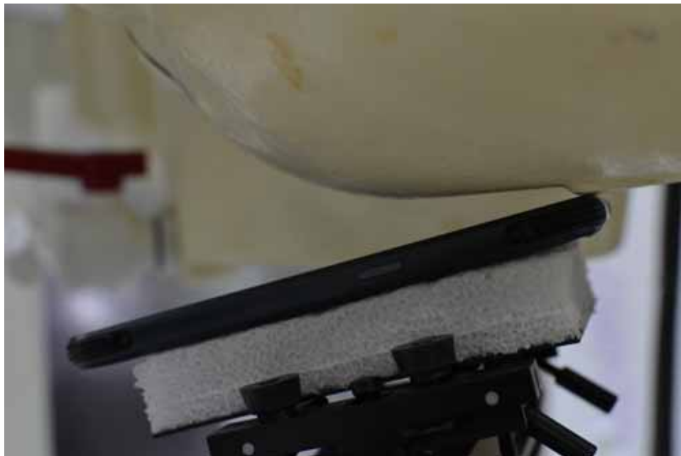
SAR Test Setup Photo 4 – Left Tilt
