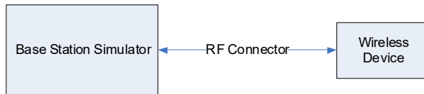
Figure 9-3 Power Measurement Setup
