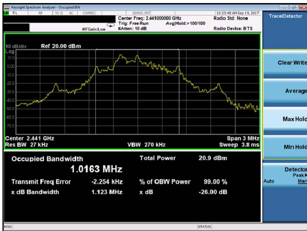
Plot 7-1. Occupied Bandwidth Plot (ANT+ – Ch. 39)
