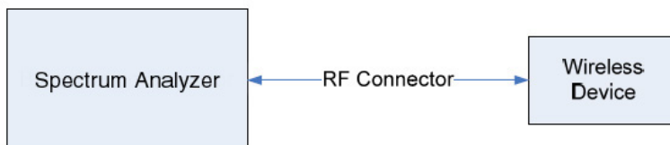
Figure 7-1. Test Instrument & Measurement Setup
