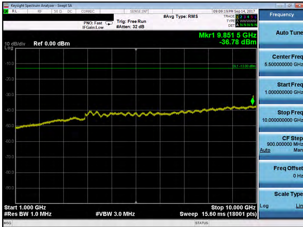
Plot 7-132. Conducted Spurious Plot (Band 13 – 5.0MHz QPSK – RB Size 1, RB Offset 0 – High Channel)
