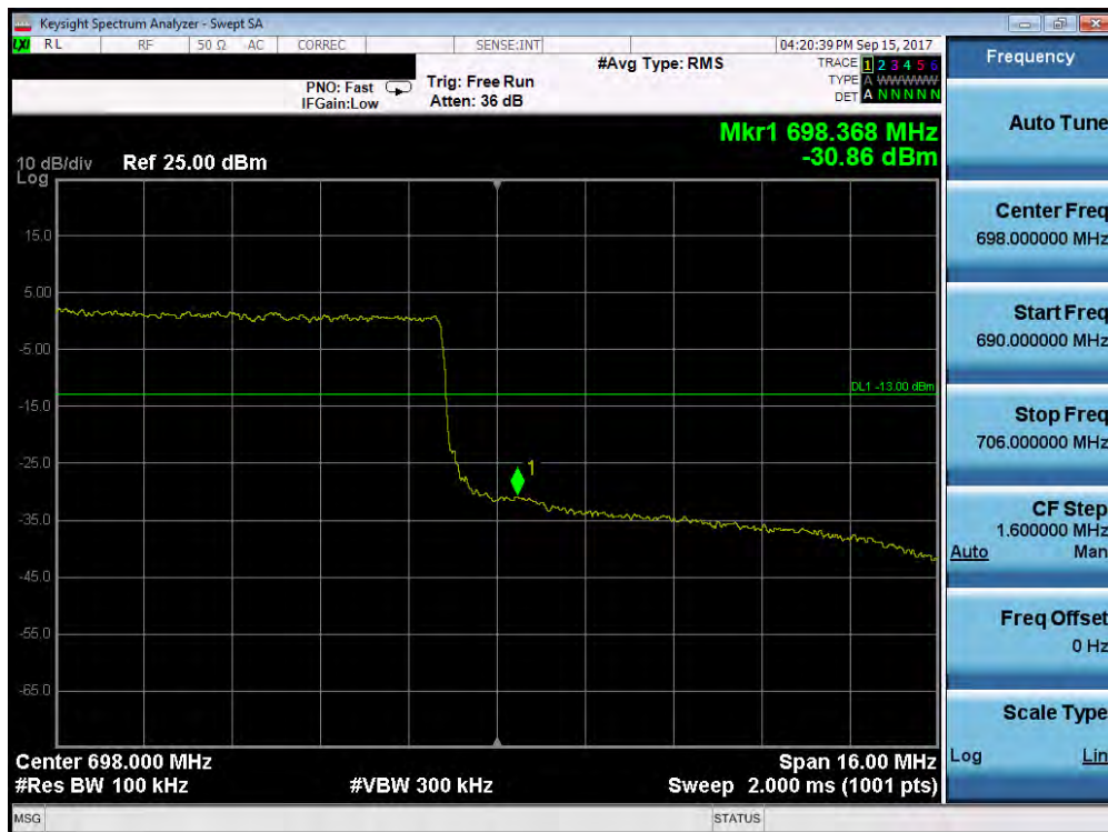
Plot 7-185. Upper Band Edge Plot (Band 71 – 20.0MHz QPSK – RB Size 100)
