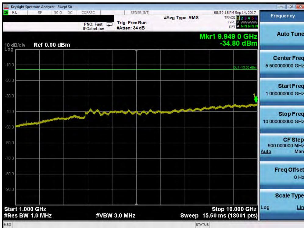
Plot 7-123. Conducted Spurious Plot (Band 12/17 – 10.0MHz QPSK – RB Size 1, RB Offset 0 – High Channel)
