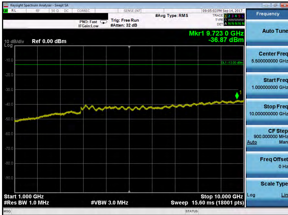
Plot 7-126. Conducted Spurious Plot (Band 13 – 5.0MHz QPSK – RB Size 1, RB Offset 0 – Low Channel)
