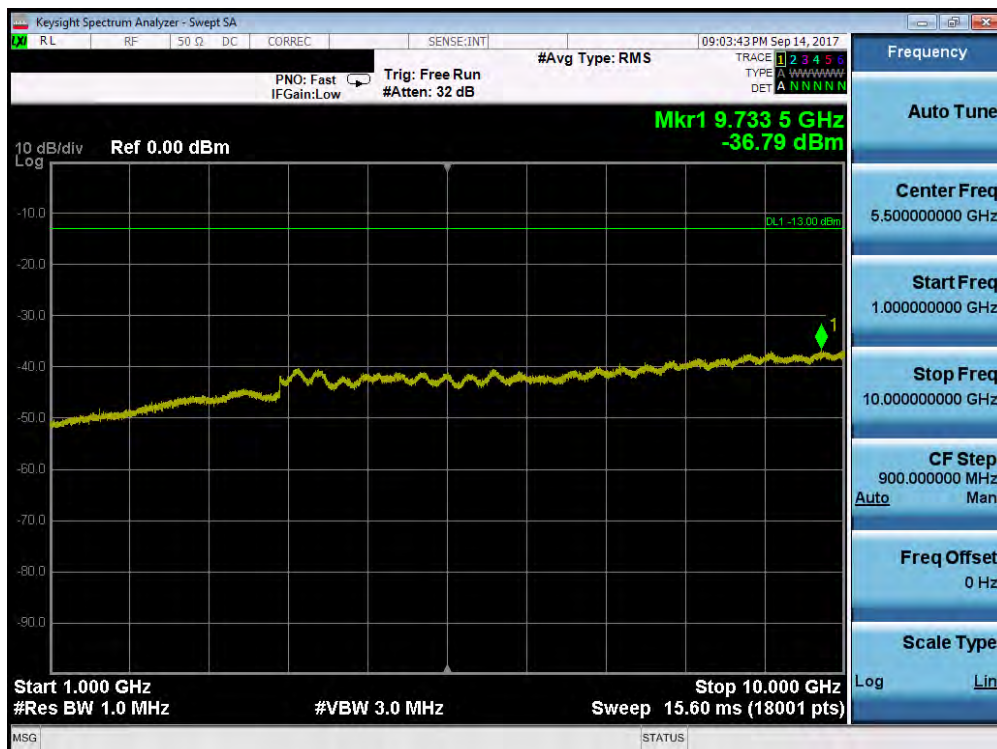
Plot 7-129. Conducted Spurious Plot (Band 13 – 5.0MHz QPSK – RB Size 1, RB Offset 0 – Mid Channel)
