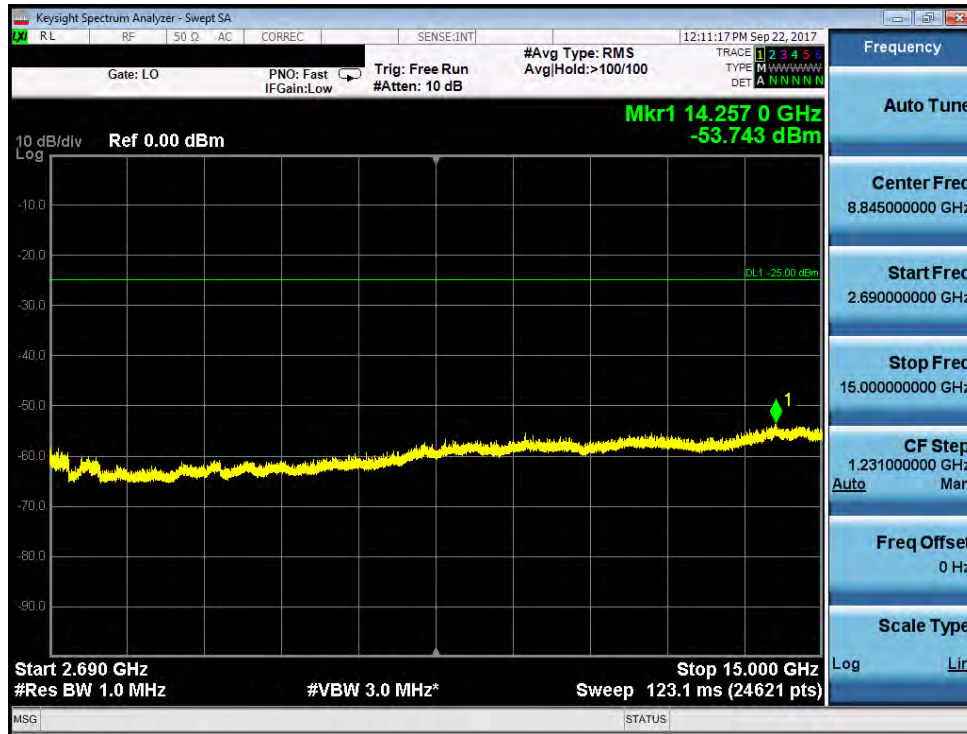
Plot 7-312. Conducted Spurious Plot (Band 41 – 20.0MHz QPSK – PCC 1/99 SCC 1/0 – Mid Channel)
