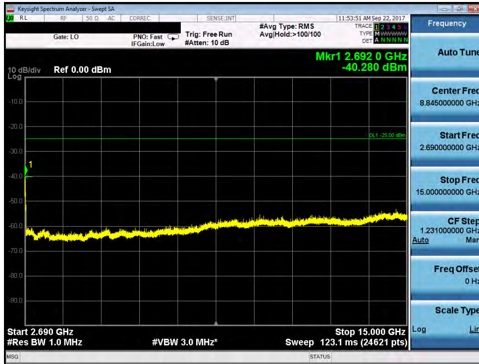
Plot 7-316. Conducted Spurious Plot (Band 41 – 20.0MHz QPSK – PCC 100/0 SCC 100/0 – Mid Channel)
