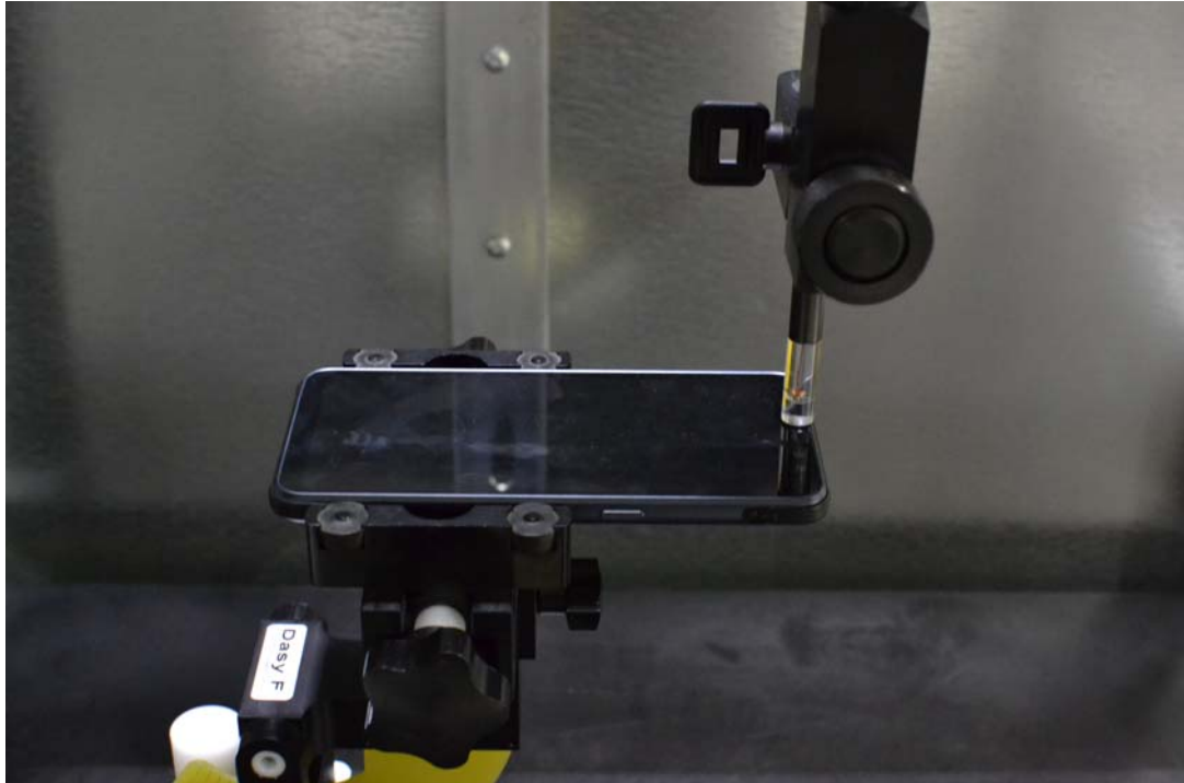
Figure 14-1 Test Setup for Wireless Device
