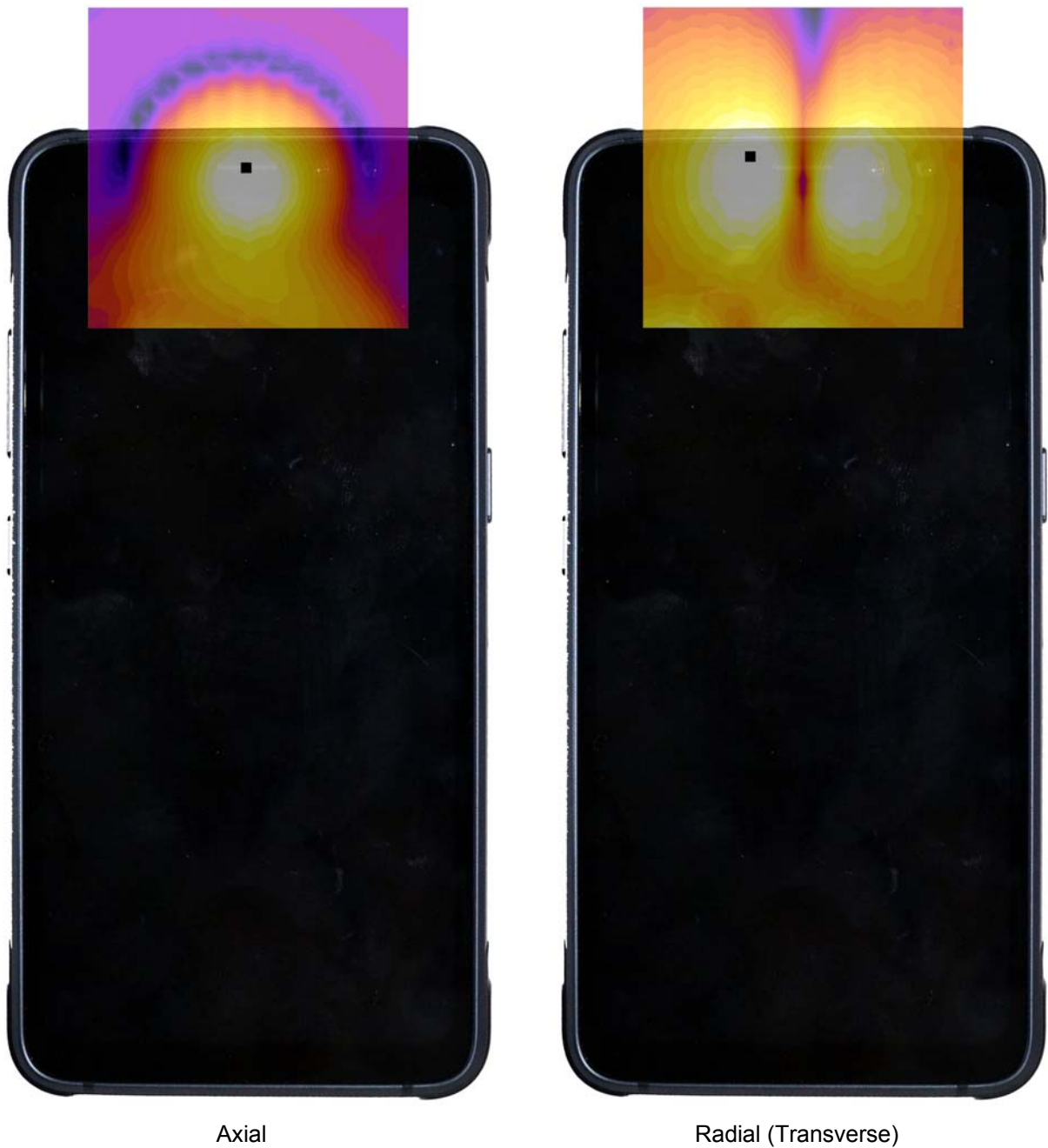
Figure 14-3 T-Coil Scan Overlay Magnetic Field Distributions
