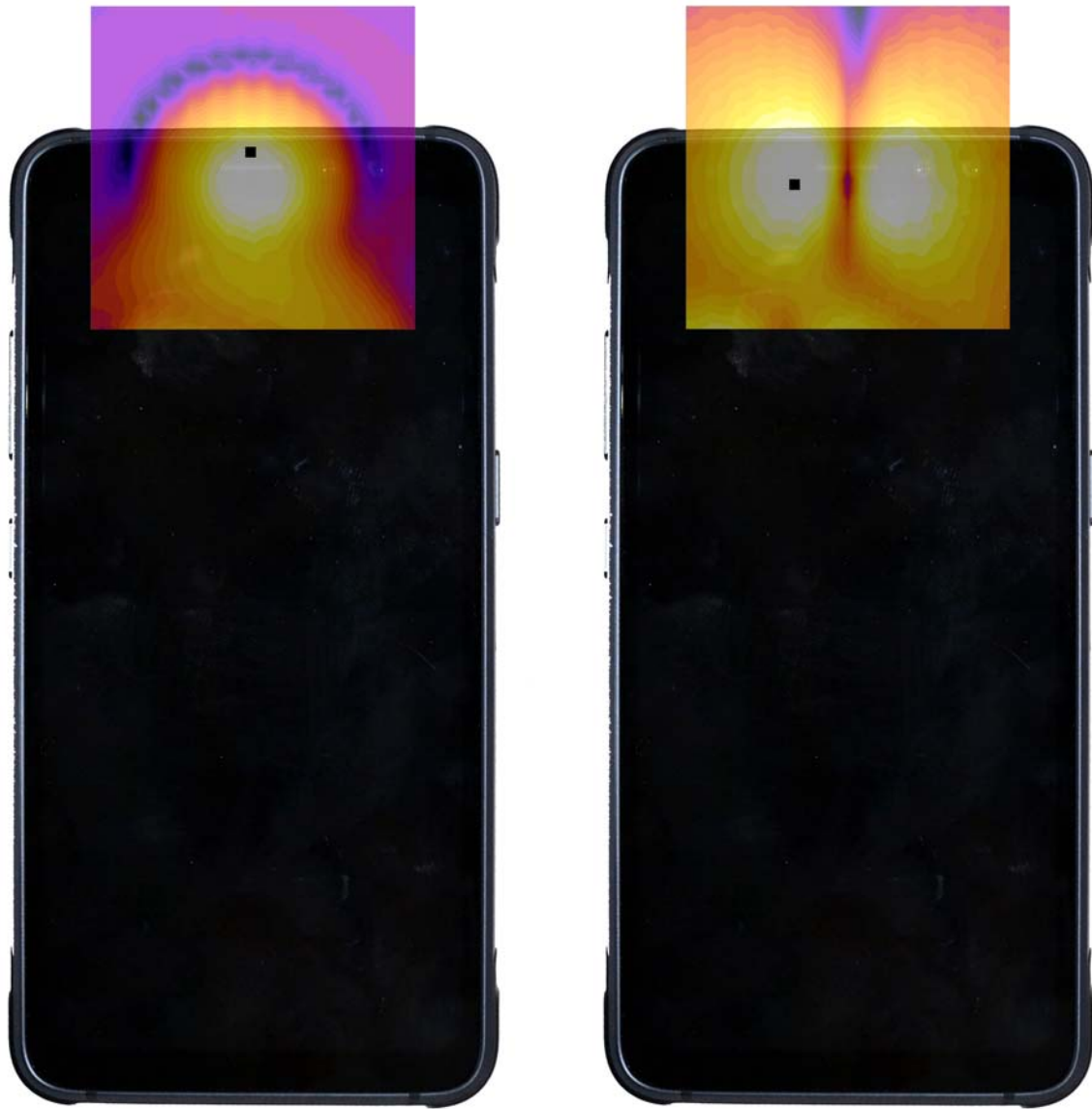
Figure 15-3 T-Coil Scan Overlay Magnetic Field Distributions
