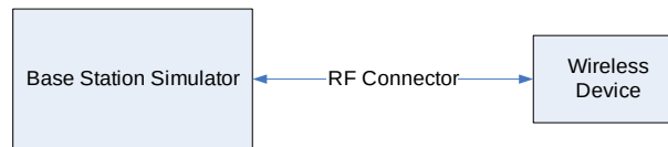
Figure 9-2 Power Measurement Setup
