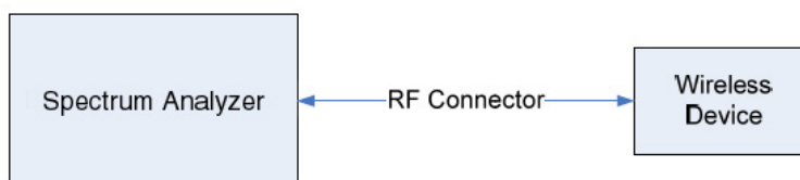
Figure 6-1. Test Instrument & Measurement Setup
