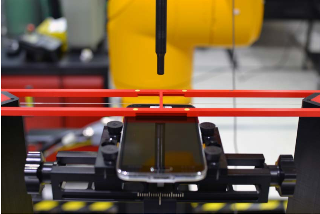
Figure 18-1 Ear Reference Point HAC Phantom Alignment
