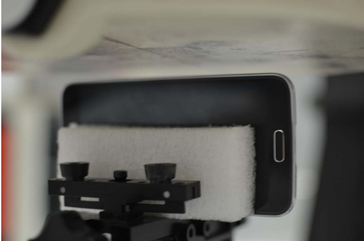
SAR Test Setup Photo 13 – Right Edge at 1.0 cm, Standard Battery Cover
