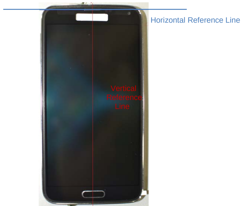
SAR Test Setup Photo 14 – Horizontal and Vertical Reference Lines
