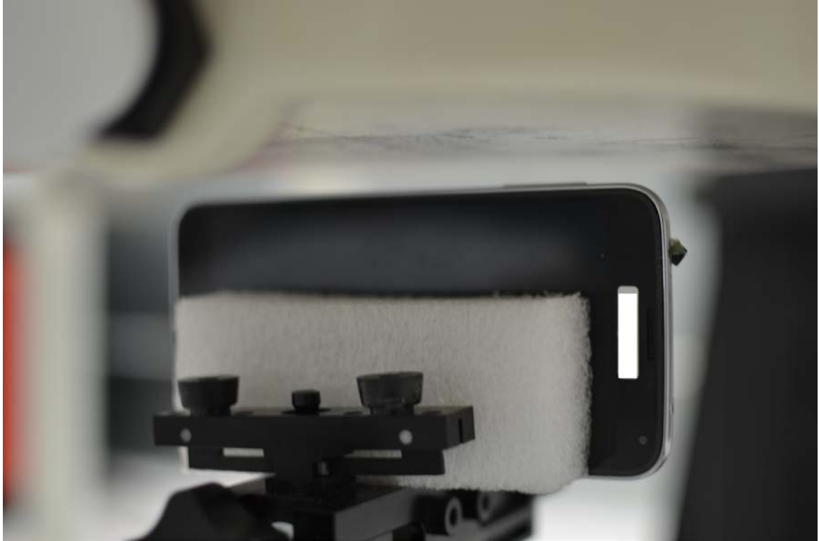
SAR Test Setup Photo 11 – Left Edge at 1.0 cm, Standard Battery Cover
