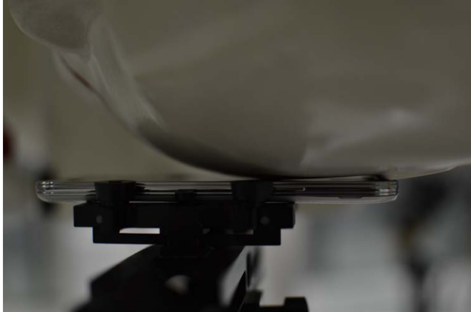
SAR Test Setup Photo 3 – Left Cheek, Standard Battery Cover
