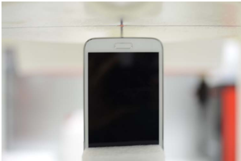
SAR Test Setup Photo 10 – Bottom Edge at 1.0 cm, Standard Battery Cover
