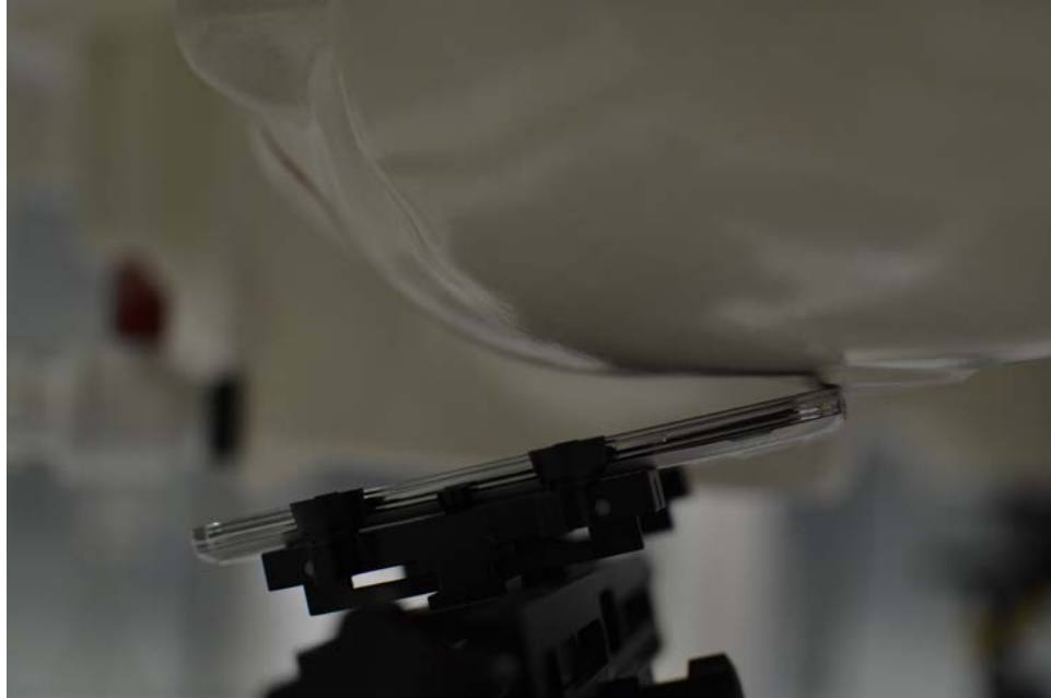
SAR Test Setup Photo 5 – Left Tilt, Standard Battery Cover
