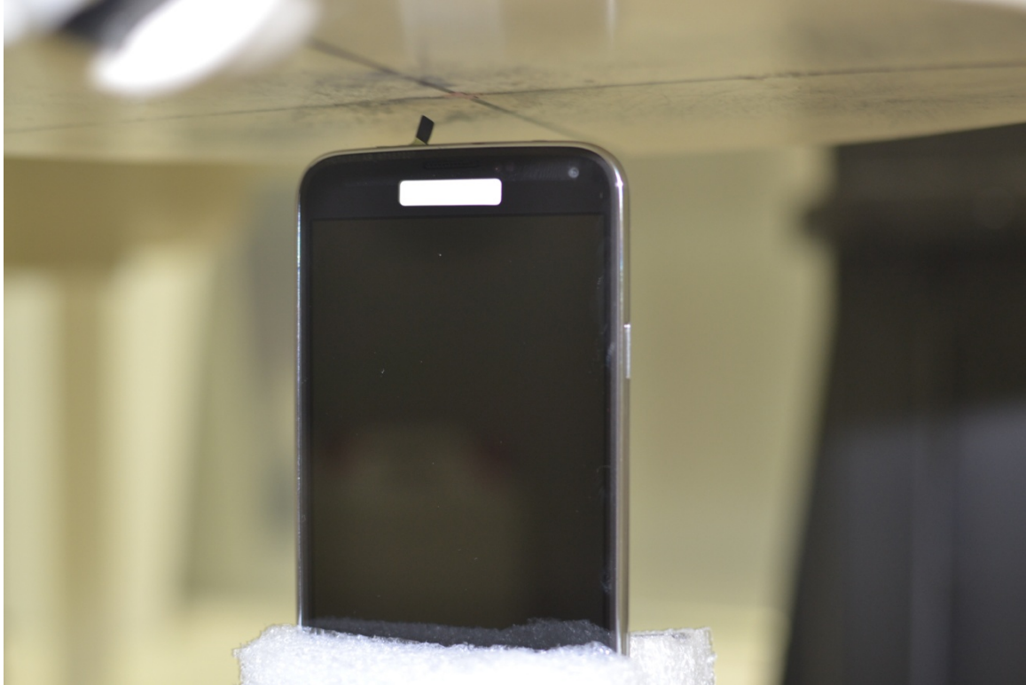
SAR Test Setup Photo 7 – Top Edge at 1.0 cm
