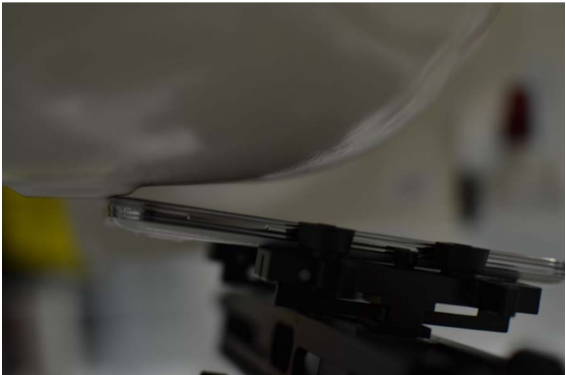
SAR Test Setup Photo 2 – Right Tilt
