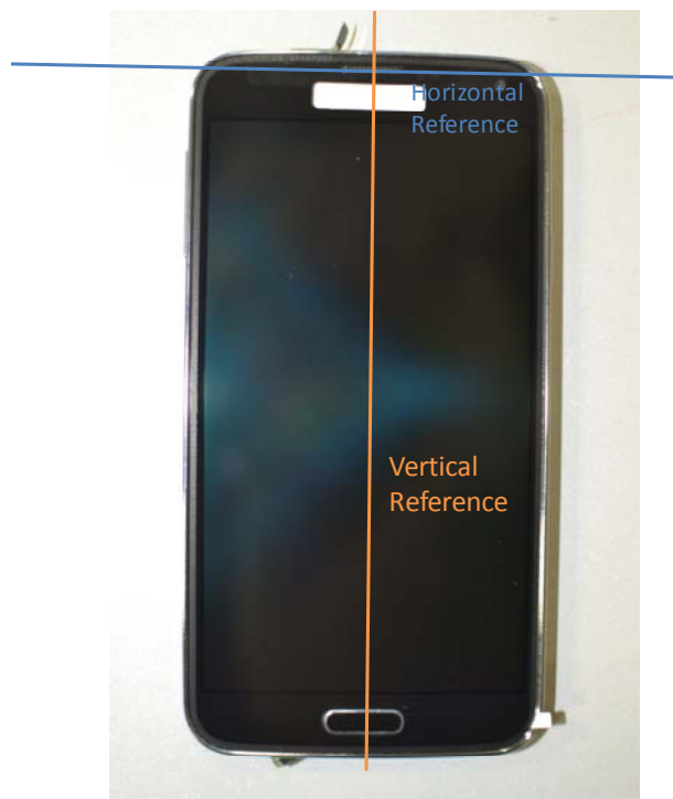
SAR Test Setup Photo 10 – Horizontal and Vertical Reference Lines
