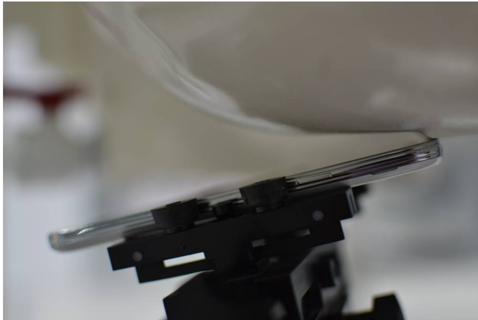
SAR Test Setup Photo 4 – Left Tilt
