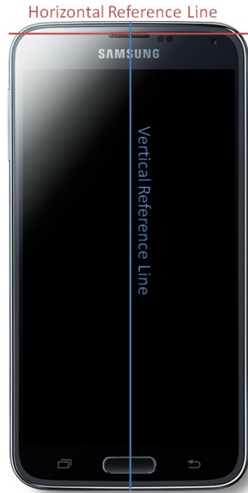
SAR Test Setup Photo 9 – Horizontal and Vertical Reference Lines
