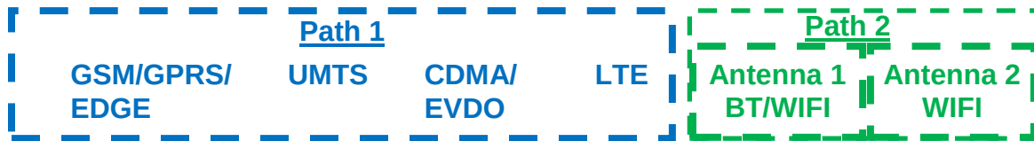
Figure 1-3 Simultaneous Transmission Paths
