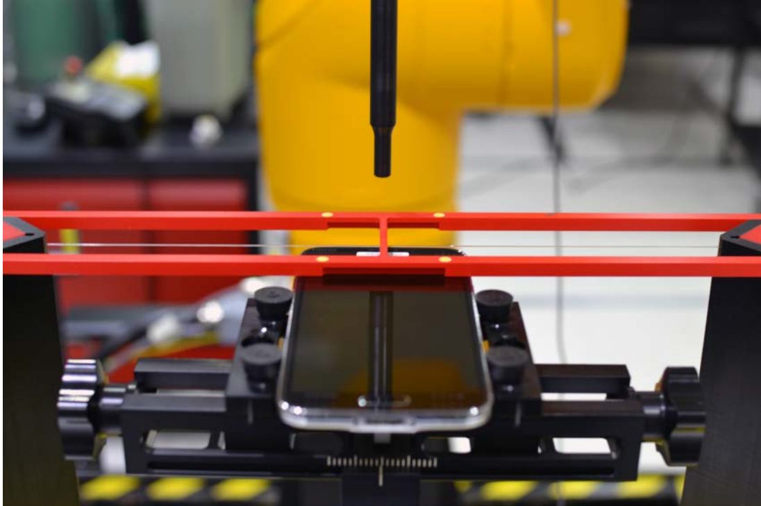
Figure 18-1 Ear Reference Point HAC Phantom Alignment
