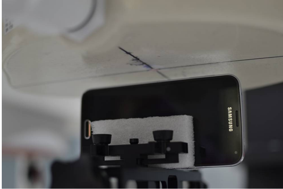
SAR Test Setup Photo 17 – Left Edge at 1.0 cm
