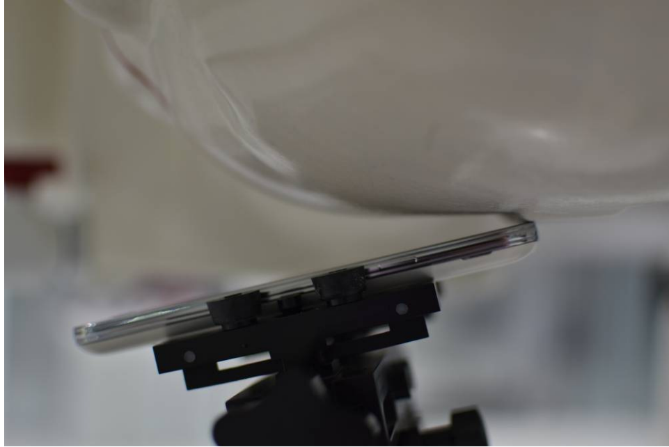
SAR Test Setup Photo 7 – Left Tilt with Wireless Charging Cover
