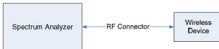
Figure 6-1. Test Instrument & Measurement Setup
