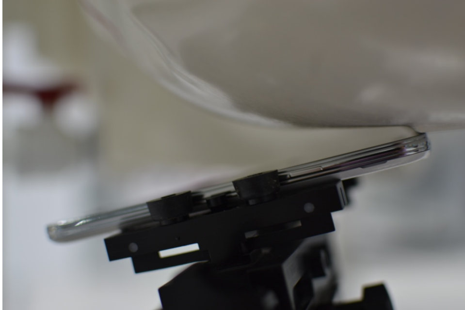
SAR Test Setup Photo 5: Left Tilt with Standard Cover
