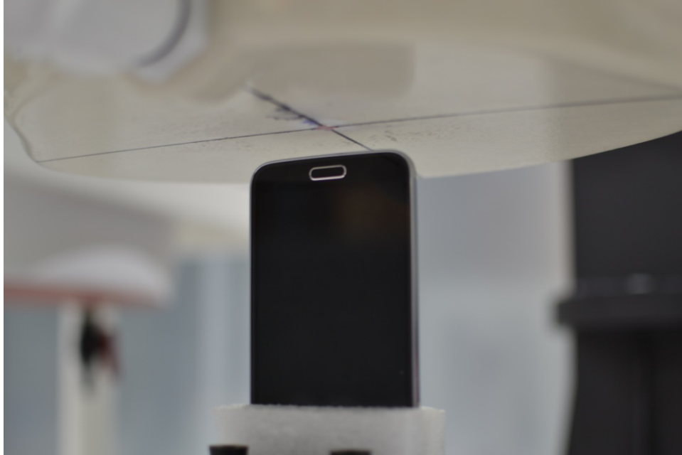
SAR Test Setup Photo 11: Bottom Edge at 1.0 cm with Standard Cover
