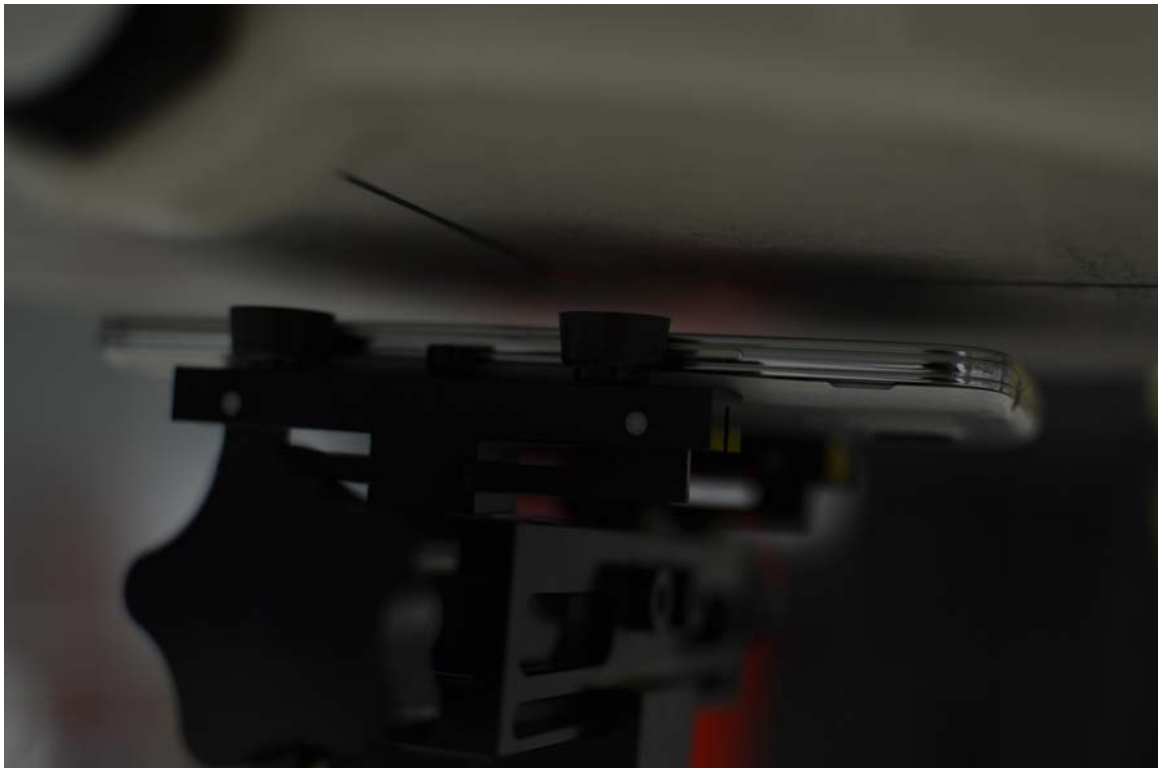
SAR Test Setup Photo 10 – Front Side, Standard Battery Cover at 1.0 cm
