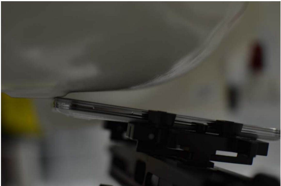
SAR Test Setup Photo 2 – Right Tilt, Standard Battery Cover
