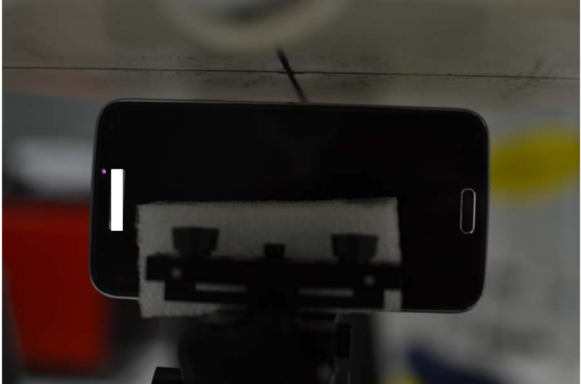
SAR Test Setup Photo 15 – Right Edge, Standard Battery Cover at 1.0 cm
