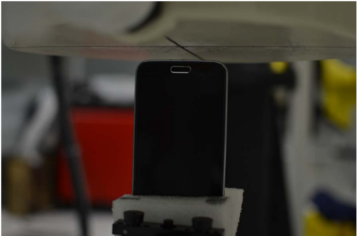
SAR Test Setup Photo 14 – Bottom Edge, Standard Battery Cover at 1.0 cm
