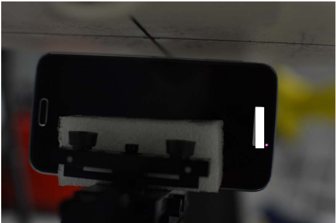
SAR Test Setup Photo 16 – Left Edge, Standard Battery Cover at 1.0 cm
