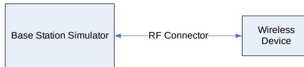
Figure 9-1 Power Measurement Setup
