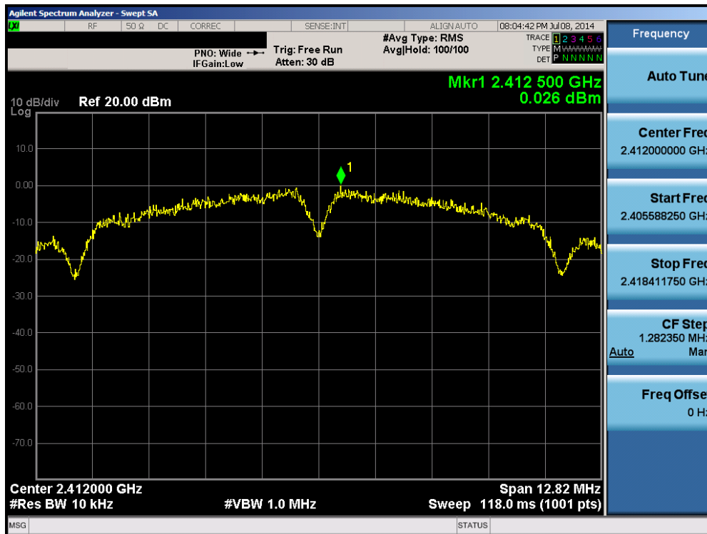
Plot 6-55. Power Spectral Density Plot (802.11b – Ch. 1)
