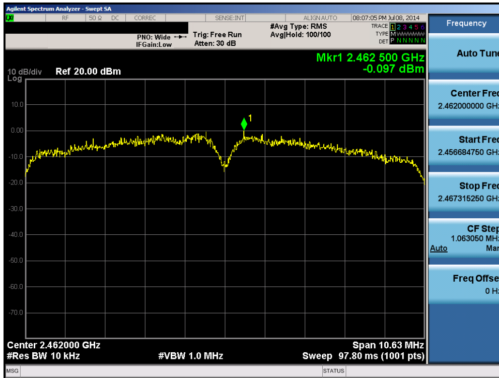
Plot 6-57. Power Spectral Density Plot (802.11b – Ch. 11)
