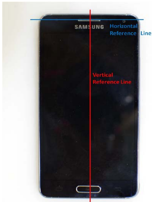
SAR Test Setup Photo 10: Horizontal and Vertical Reference Lines
