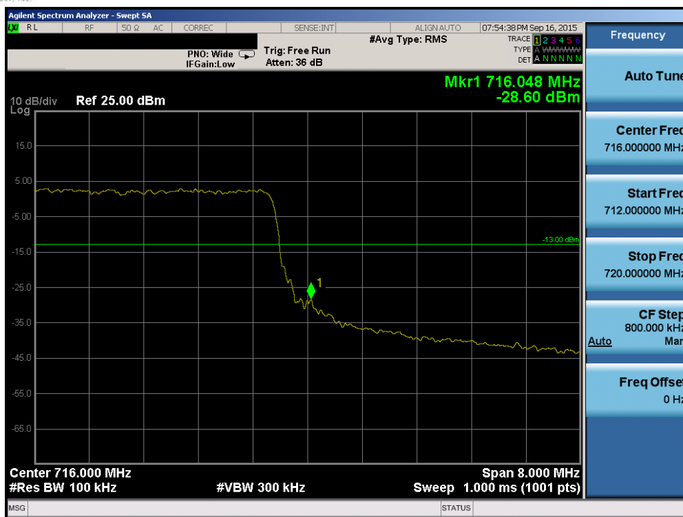
Plot 6-103. Upper Band Edge Plot (Band 12/17 – 10.0MHz QPSK – RB Size 50)
