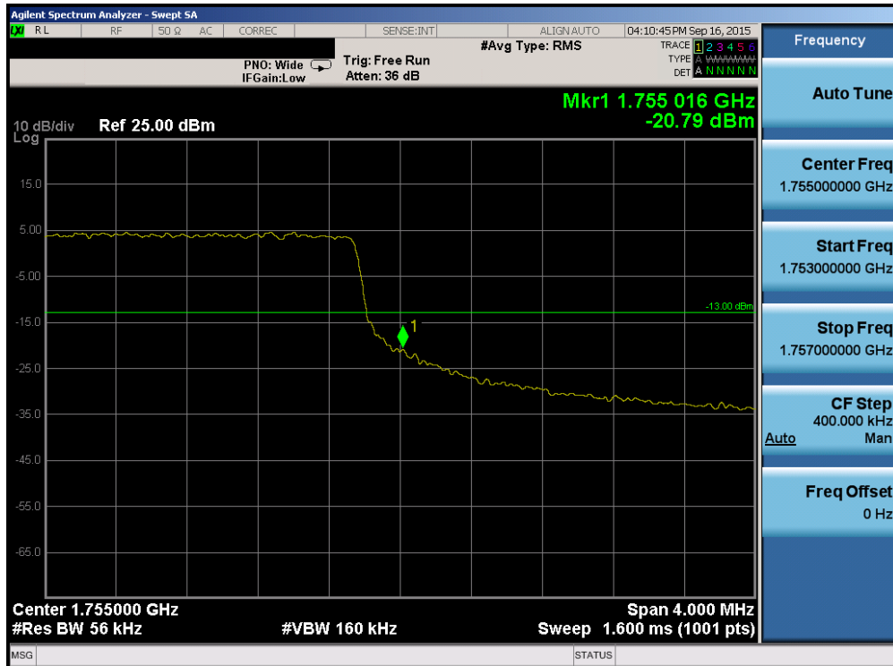
Plot 6-138. Upper Band Edge Plot (Band 4 – 5.0MHz QPSK – RB Size 25)
