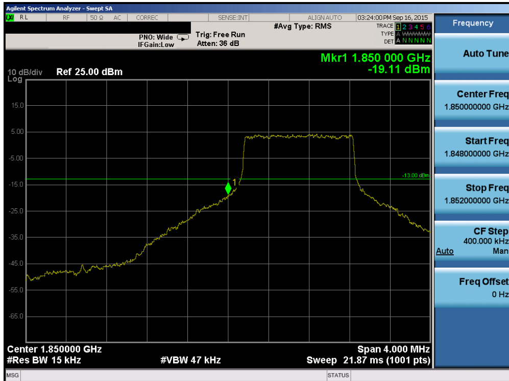
Plot 6-152. Lower Band Edge Plot (Band 2 – 1.4MHz QPSK – RB Size 6)
