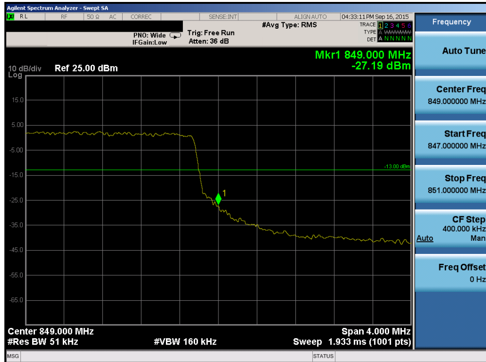
Plot 6-124. Upper Band Edge Plot (Band 5 – 5.0MHz QPSK – RB Size 25)
