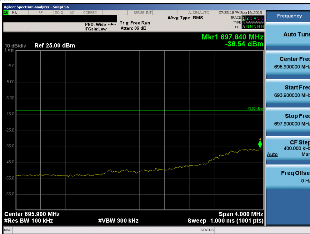
Plot 6-91. Lower Extended Band Edge Plot (Band 12 – 1.4MHz QPSK – RB Size 6)
