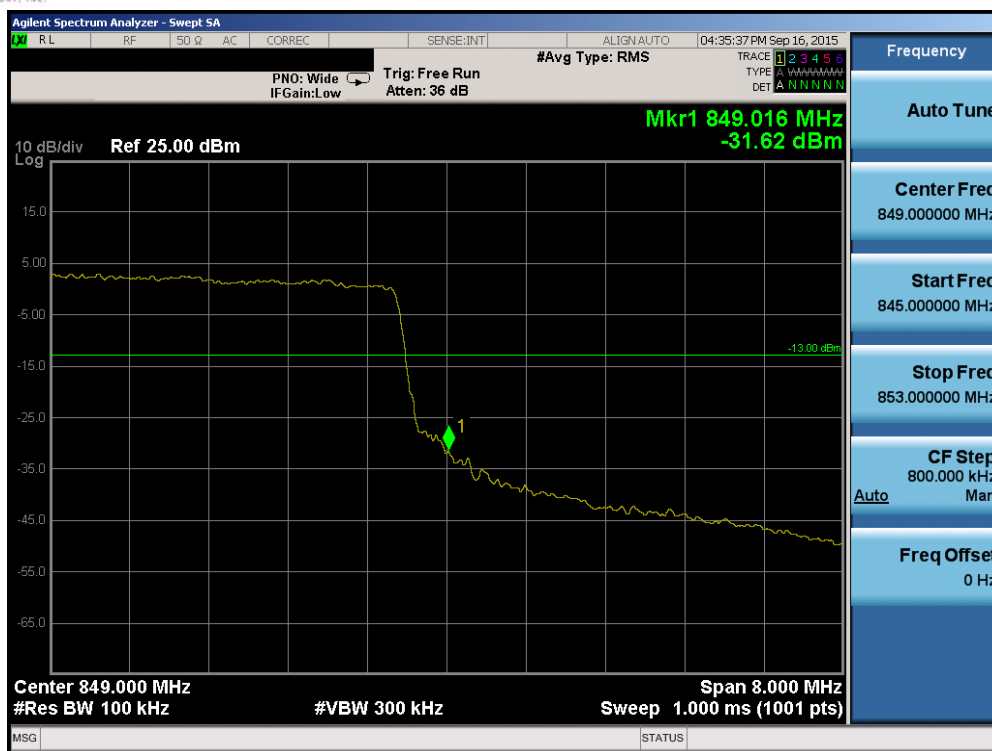
Plot 6-127. Upper Band Edge Plot (Band 5 – 10.0MHz QPSK – RB Size 50)
