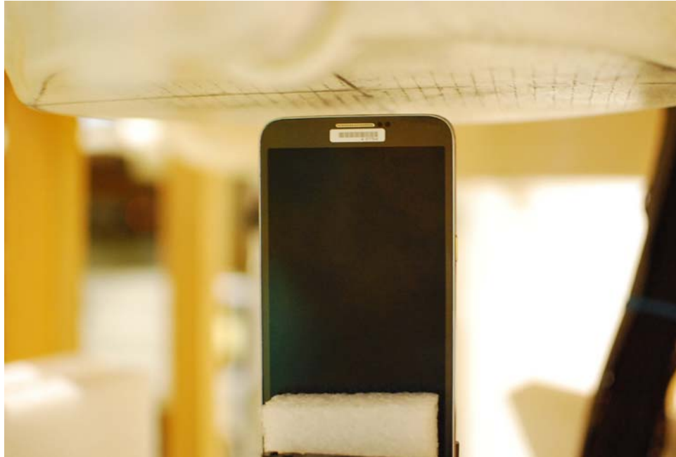
SAR Test Setup Photo 7: Top at 1.0 cm
