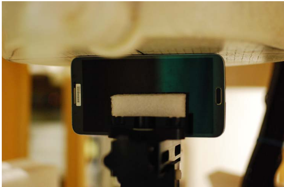
SAR Test Setup Photo 14: Right at 1.0 cm
