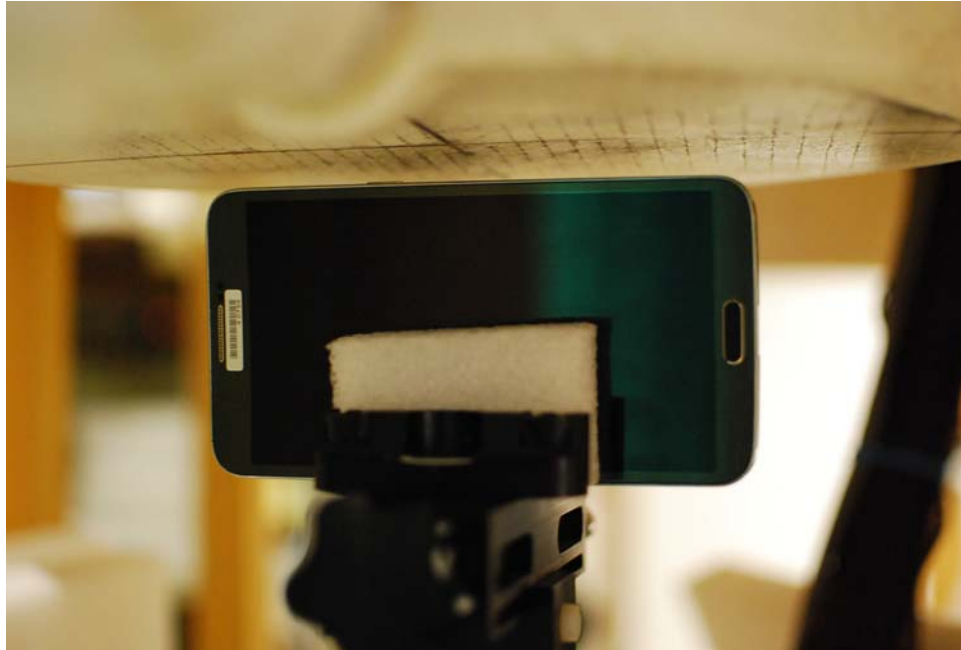
SAR Test Setup Photo 9: Right at 1.0 cm
