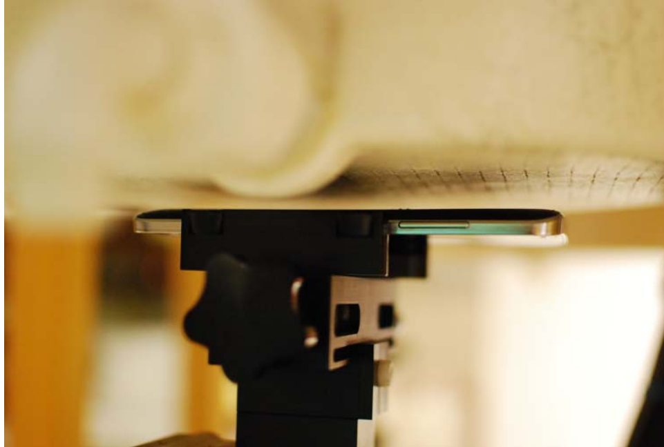
SAR Test Setup Photo 5: Back at 1.0 cm
