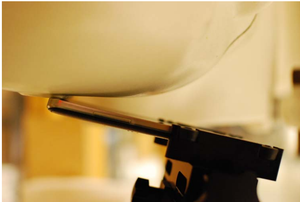
SAR Test Setup Photo 2: Right Tilt
