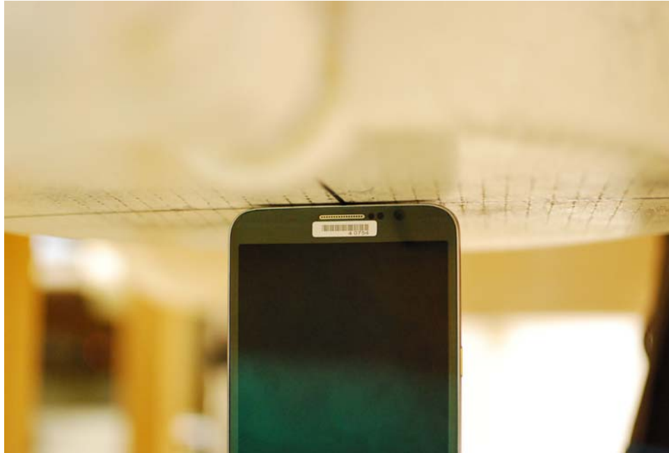
SAR Test Setup Photo 13: Top at 0.0 cm
