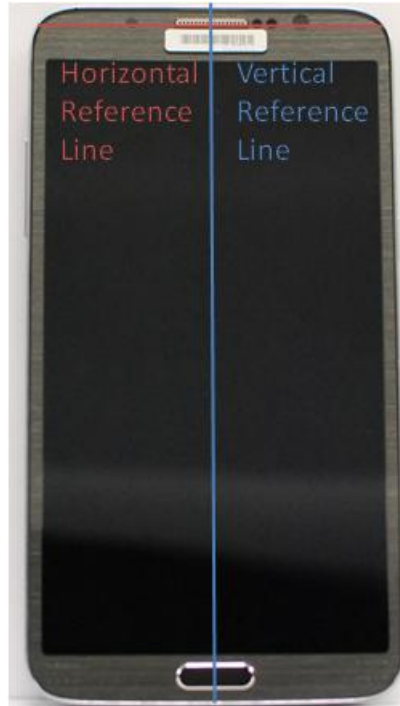
SAR Test Setup Photo 15: Reference Lines
