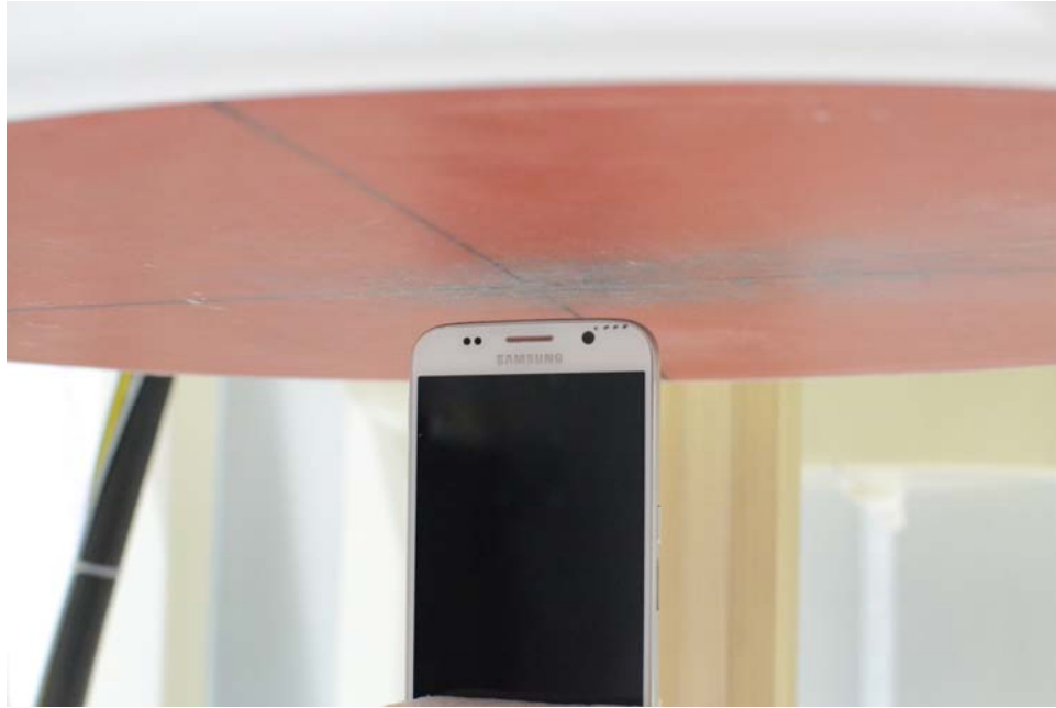
SAR Test Setup Photo 7: Top at 1.0 cm
