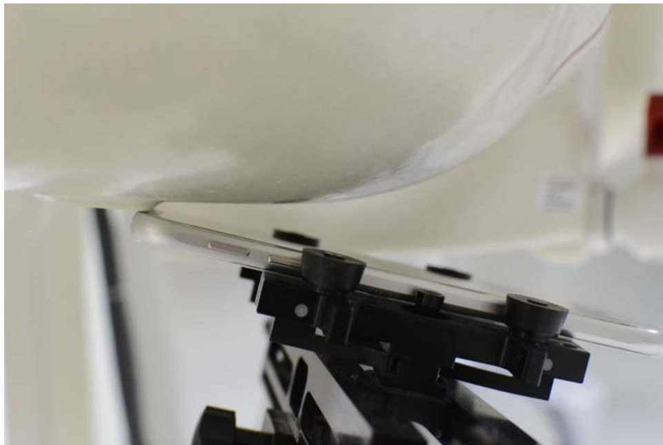
SAR Test Setup Photo 2: Right Tilt
