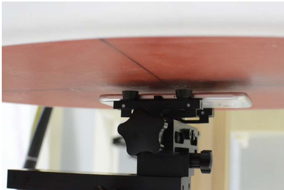
SAR Test Setup Photo 6: Front at 1.0 cm
